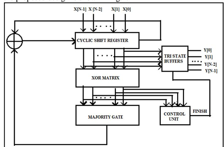
Fig.2 Internal block diagram of MLDD.
