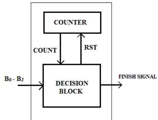
Fig 5. Block diagram of control unit.
