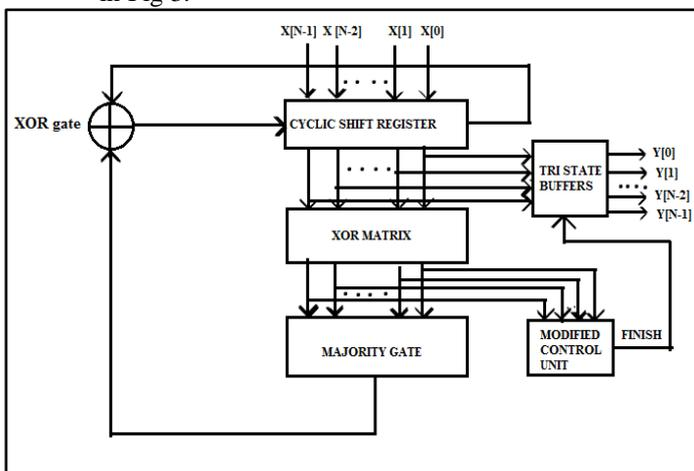
Fig.3. Internal block diagram of high Performance MLDD.
