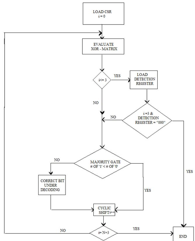
Fig.4. Flow chart of MLDD algorithm.
