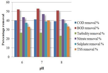
Fig. 6 Effect of pH on anaerobic treatment efficiency of synthetic leachate
