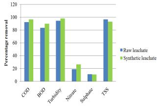
Fig. 4 Removal efficiency of raw and synthetic leachate upon Fenton treatment
