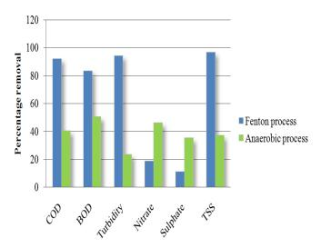
Fig. 8 Efficiency of Fenton and anaerobic process in treating mature landfill leachate
