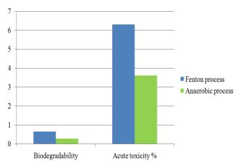
Fig. 9 Biodegradability and acute toxicity of Fenton and anaerobic treated mature landfill leachate
