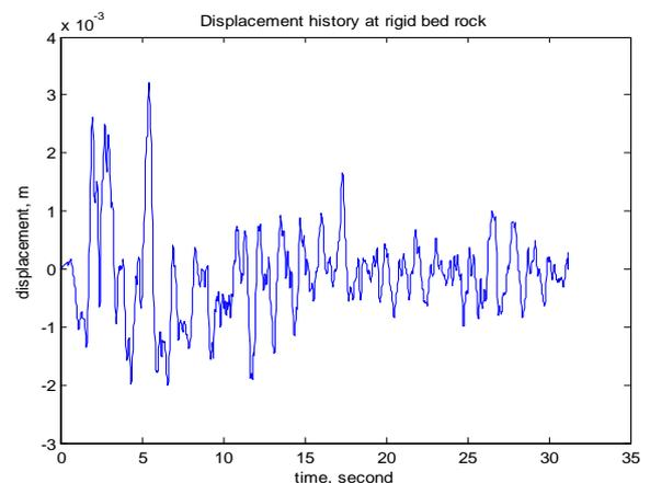
Figure 4: Displacement at rigid bed rock with time.
