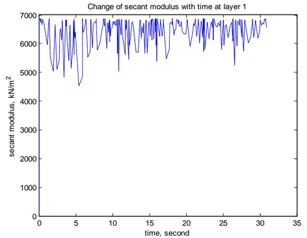
Figure 8: Change of secant modulus with time in a layer just below the surface layer.
