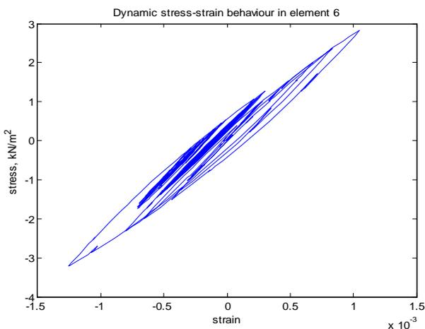
Figure 7: Dynamic stress-strain behaviour in an intermediate layer.
