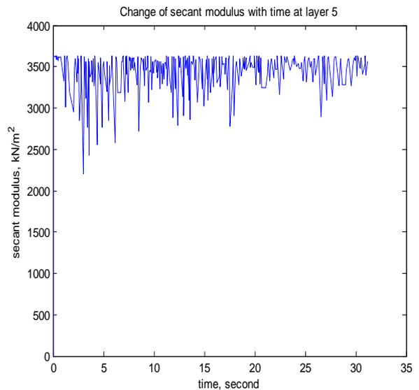
Figure 9: Change of secant modulus with time in an intermediate layer.
