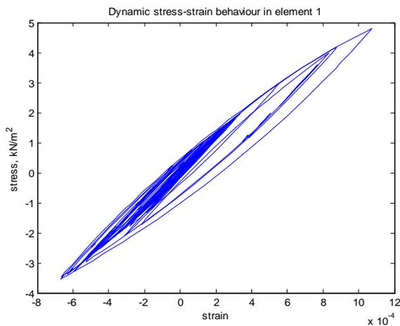
Figure 6: Dynamic stress-strain behaviour in a layer just below the surface layer.
