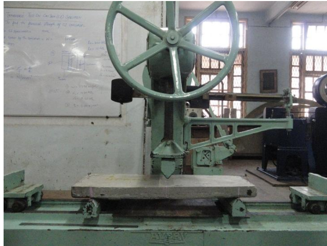
Slab specimen under one point flexural loading system (Ducts filled with resins)
