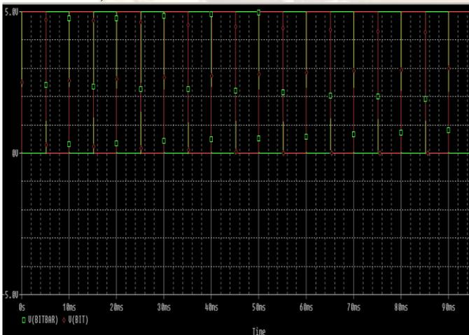
Figure 7: Simulation result of 6t SRAM cell
