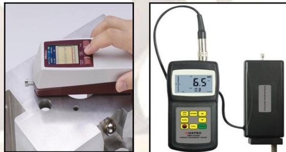
Fig 12 Surface Roughness Tester
