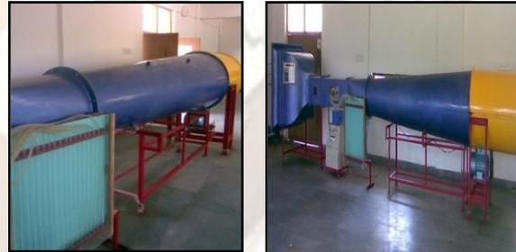
Fig 8 Diffuser Section
