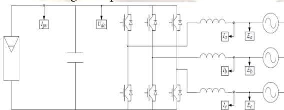
Fig3: Proposed Electrical Scheme
