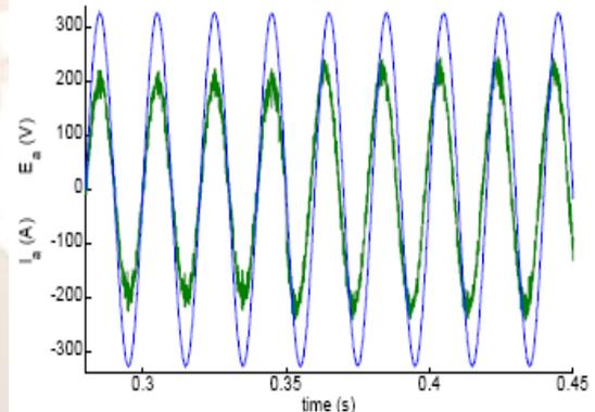
Fig. 12: Inverter response to a step in reactive power reference in  $t=0.35s$ .
