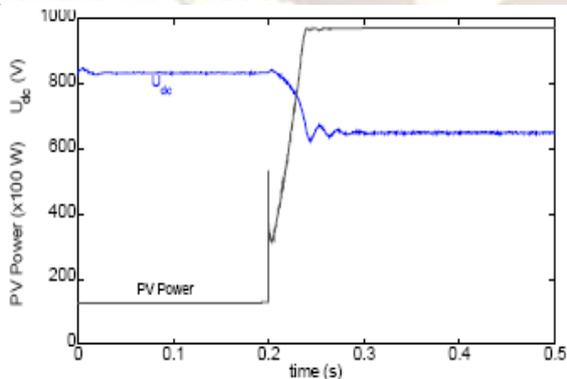
Fig 10: System response to an irradiance step  $t=0.2$
