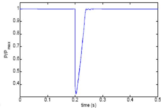
Fig11: System response to an irradiance step  $t=0.2$  sec
