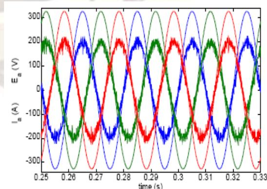
Fig. 13: Inverter behavior in operation at unity power factor
