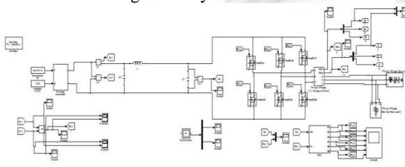
Fig 9: Simulink block diagram of photovoltaic system with MPPT controller
