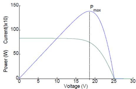
Fig4: Module power and current Vs voltage
