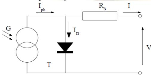
Fig1: Equivalent circuit of PV Cell
