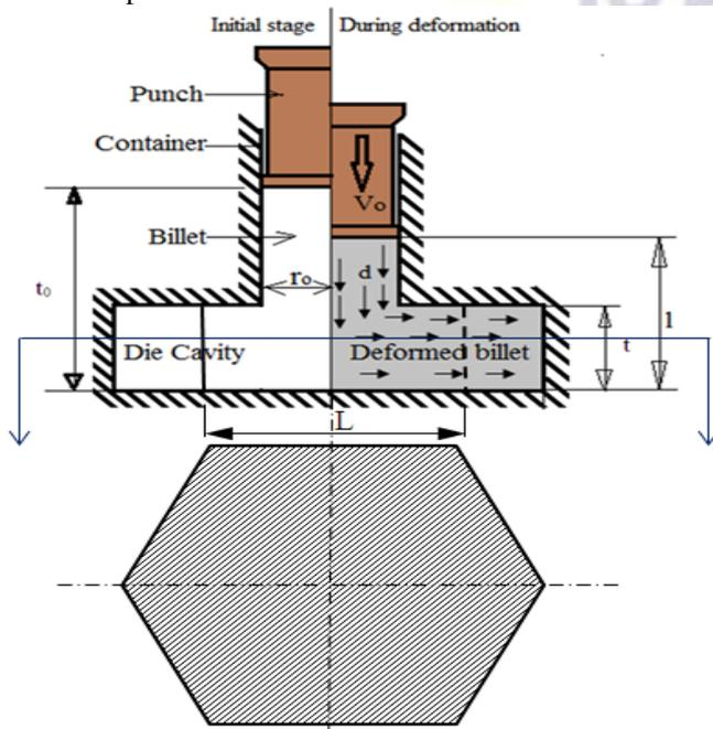
Figure 1. The schematic illustration of the lateral extrusion process and die parameters.
