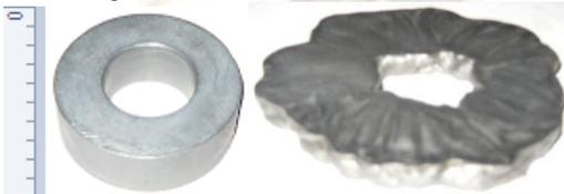
Figure 4. Lead specimen, before and after ring test.
