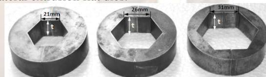
(a) Hexagonal lateral extrusion die with t=20mm.
