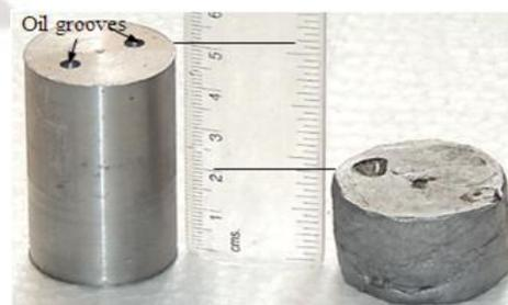
Figure 2. Shape of specimen before and after compression test.
