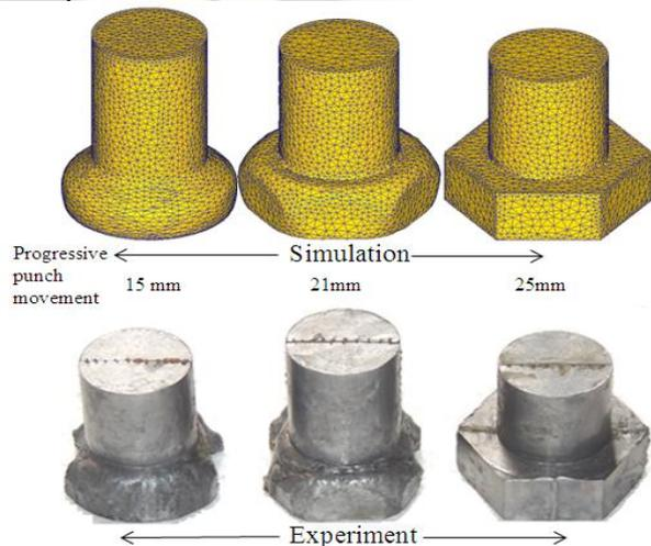
Figure 10. Die filling at different punch movement
