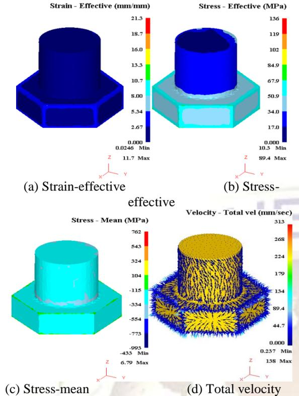
Figure 7. Stress, strain and total velocity of hexagonal headed with round shaft.
