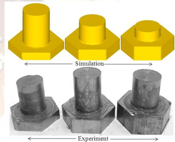
(c)Length of side=31mm and thickness, t= 10, 15 and 20mm
