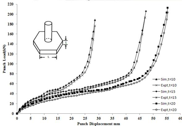
(c) Variation of punch load for 31 mm side of hexagonal head.
