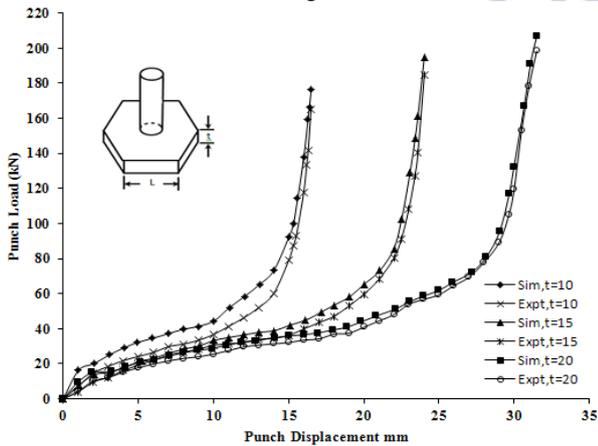
(b) Variation of punch load for 26 mm side of hexagonal head.
