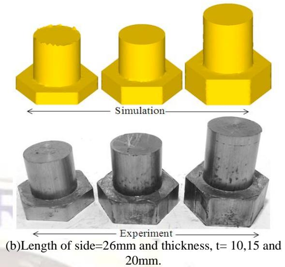
(b)Length of side=26mm and thickness, t= 10,15 and 20mm.
