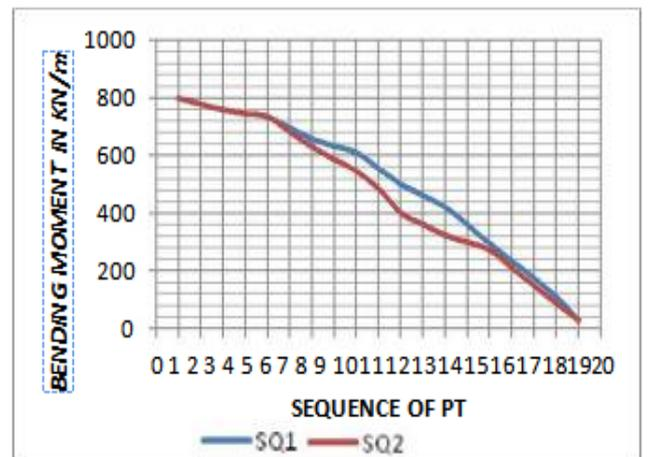
Graph-10 Comparison of bending moment in between sequential pre-stress pattern 1 and pattern 2 in X-direction for beam number 6.
