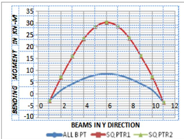
Graph-7 Comparison of bending moment in between immediate pre-stressing and sequential patterns for transfer case 1.0(DL+PT) in Y-dir.
