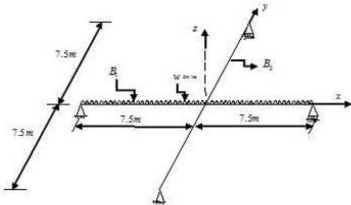
Fig. 3 Simply supported cross beam.
