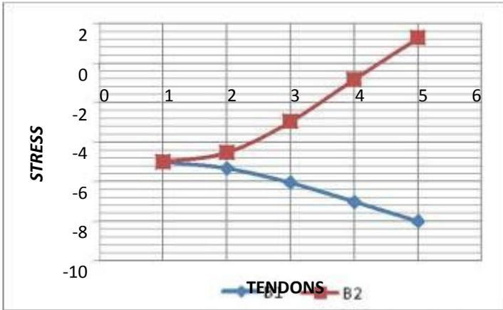
Graph-4 Comparison of flexural stress on top fibre in transfer case 1.0(DL+PT)
