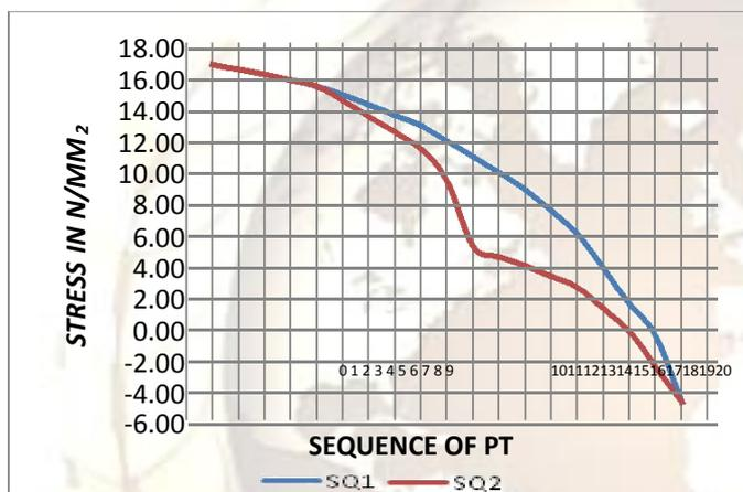
Graph-13 Comparison of bending stress in between sequential pre-stress pattern 1 and pattern 2 in Y-direction for beam number 17.
