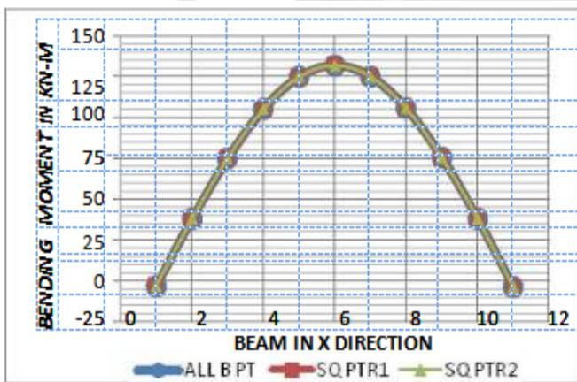
Graph-8 Comparison of bending moment in between immediate pre-stressing and sequential patterns for transfer case 1.0(DL+PT) in X-dir.
