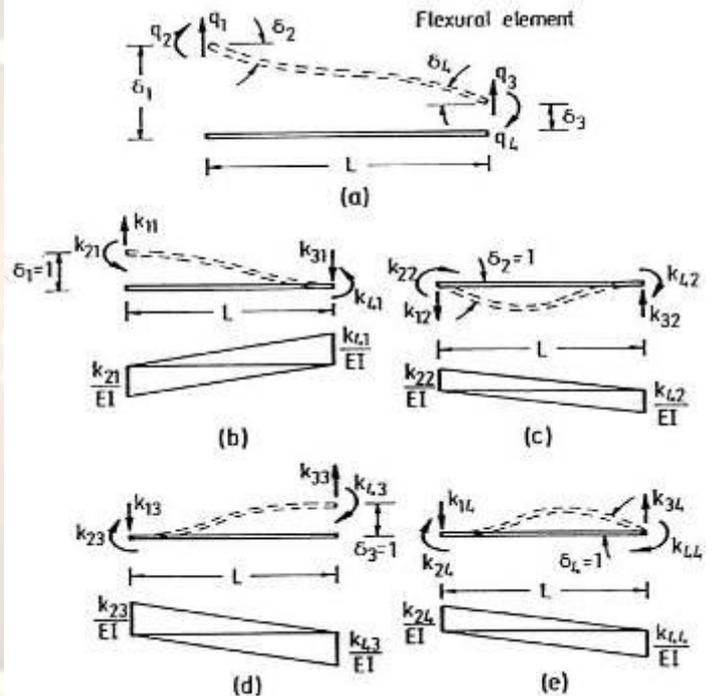
Fig.2 Beam element stiffness matrix
