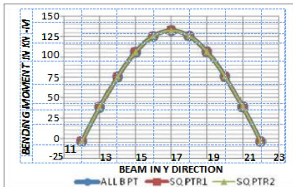
Graph-9 Comparison of bending moment in between immediate pre-stressing and sequential patterns for transfer case 1.0(DL+PF) in Y-dir.
