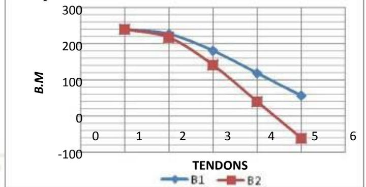
Graph-1. Comparison between bending moment of B1 and B2 beam in transfer case 1.0(DL+PT).
