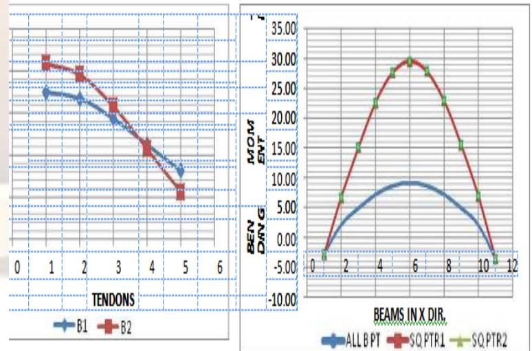
Graph-3 Comparison between bending moment of B1 and B2 beam in service case 1.0(DL+LL+PT). Graph-6 Comparison of bending moment in between immediate pre-stressing and sequential patters for transfer case 1.0(DL+PT) in X-dir.
