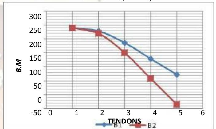
Graph-2 Comparison between bending moment of B1 and B2 beam in transfer case after all losses 1.0(DL+PT) (-ve) sig. Indicate compressive stress.
