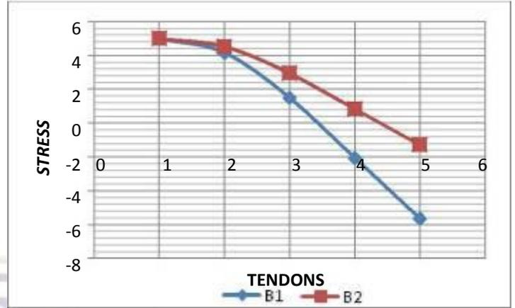
Graph-5 Comparison of flexural stress on bottom fibre in transfer case 1.0(DL+PT)
