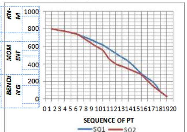
Graph-11 Comparison of bending moment in between sequential pre-stress pattern 1 and pattern 2 in Y-direction for beam number 17.
