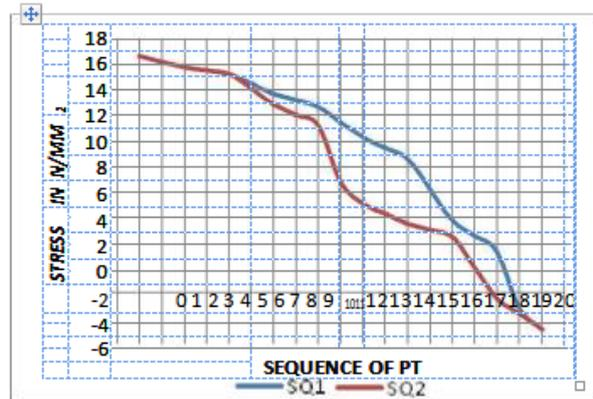
Graph-12 Comparison of bending stress in between sequential pre-stress pattern 1 and pattern 2 in X-direction for beam number 6.
