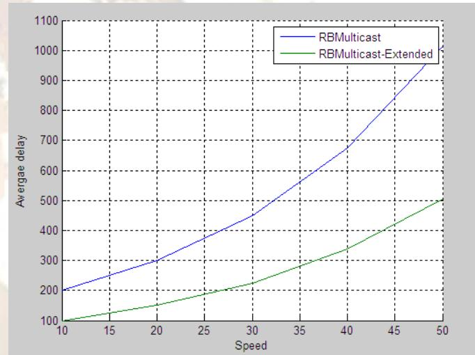
The delay increases faster in RBMulticast compared to our approach as the speed of movement increases.
