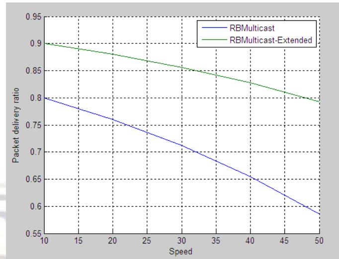
The packet delivery ratio drops faster in RBMulticast compared to our approach as speed of movement of node increases.
