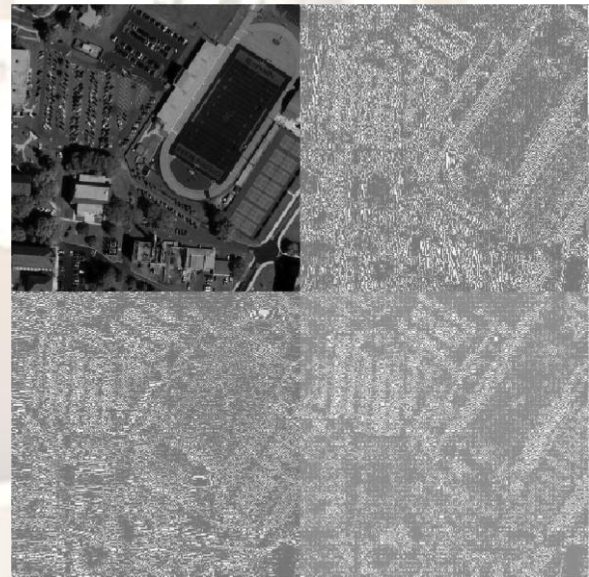
Fig. 2. LL, LH, HL, and HH subbands of a satellite image obtained by using DWT.
