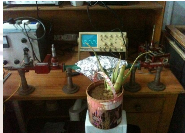
Fig. 4. Microwave setup for exposure of Aloe Vera leaf to microwaves.
