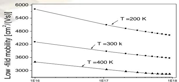
Fig 8. Changes the electron mobility Function in terms of electron concentration in bulk InN at the different Temperature
