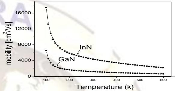
Fig 6. Changes the electron mobility Function in terms of temperature in bulk GaN and InN at the electron concentration 10<sup>16</sup> (cm<sup>-3</sup>).
