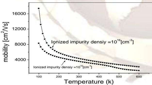
Fig 5. Changes the electron mobility Function in terms of temperature in bulk InN at the different electron concentration.
