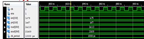
Fig: V.III Simulation results of rectangular to polar conversion
