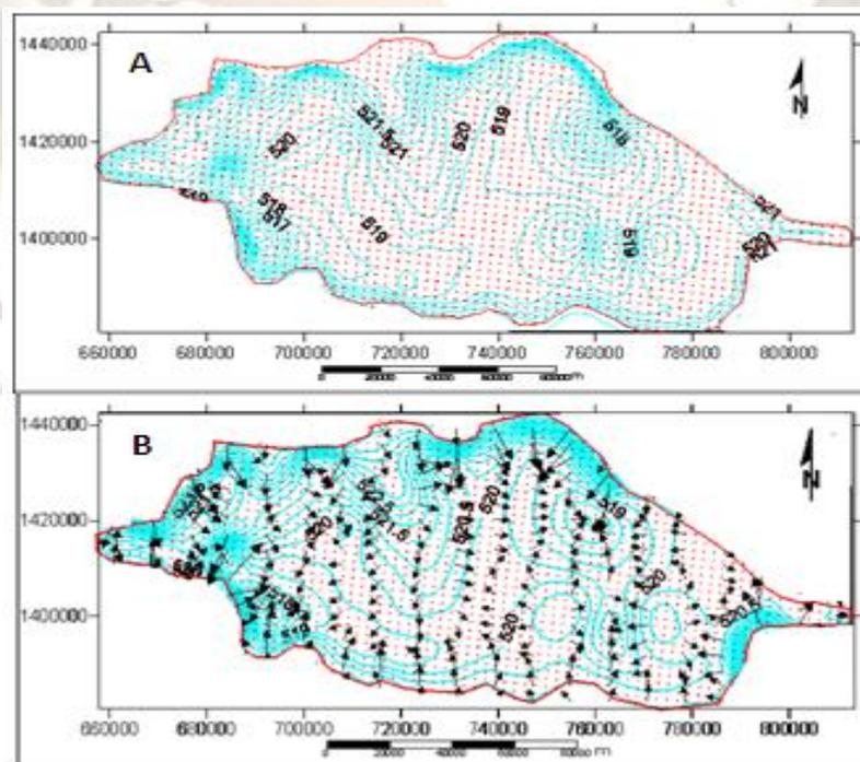
**Fig. 4. Distribution of initial head (A) and simulated head with flow direction (B).**
