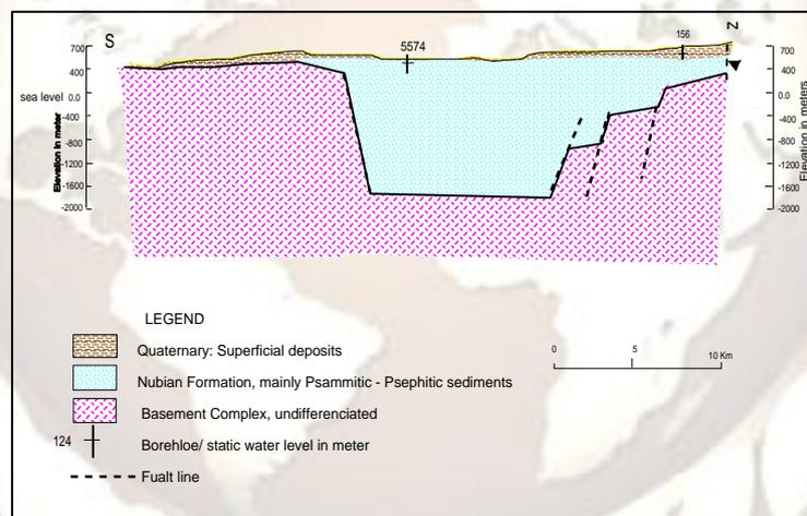
Fig.2 Schematic geological cross-section through the Model Domain
