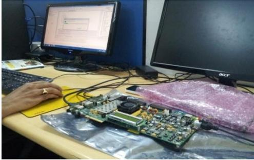
Fig.8 KINTEX7 FPGA Module Setup
