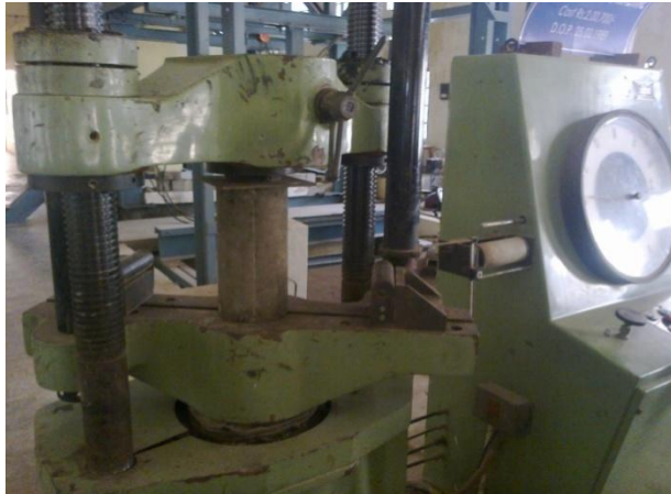
Fig 6: cylindrical compressive strength of concrete testing setup
