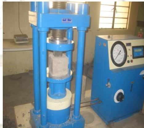
Fig 4: compressive strength of cement testing setup
