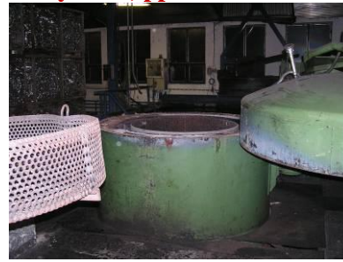
Pic. 2. A Balzer-type oven.
