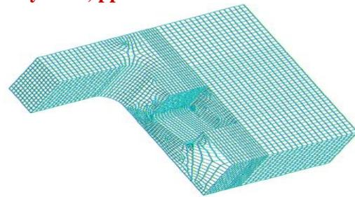
Fig - 3.18: Submodel in hyper mesh
