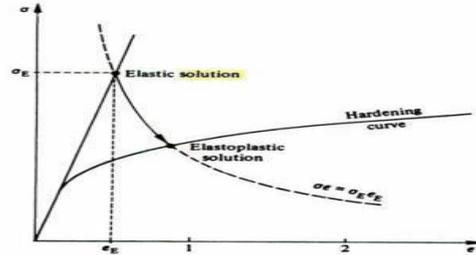
**Fig – 3.20 Stress-strain (hardening) curve**
