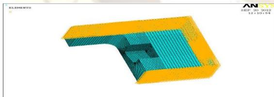
Fig – 3.13 Submodel along with new refined mesh
