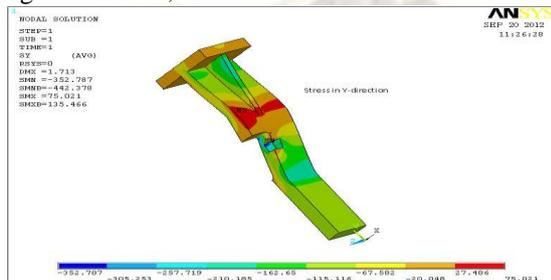
FIG – 3.6 : Stress in Y- Direction
