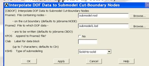
Here the node file is provided as input and the loads at the top and bottom surfaces of the submodel are interpolated from the full model. All the loads are interpolated as degree of freedom constraints and the load file for the first load step is written with the name '**submodel1.lob**'.
