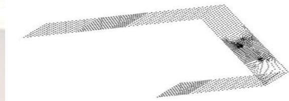
FIG – 3.19: Nodes of the submodel
