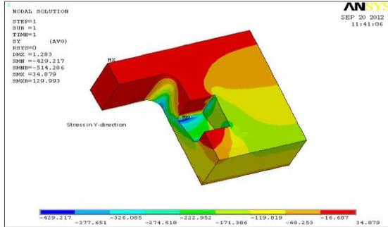
FIG – 3.11 : Stress in Y- Direction
