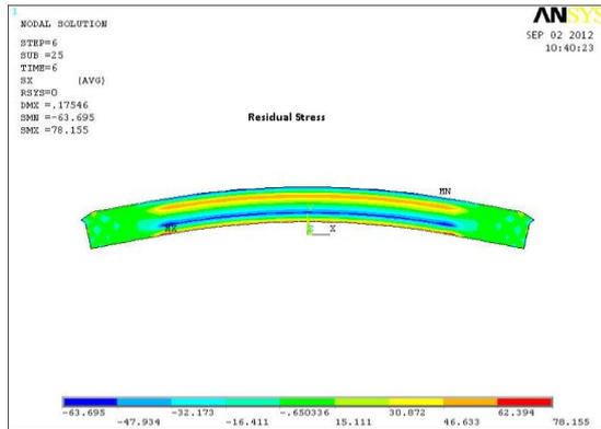
Fig – 2.7: At load 0N Residual stress
