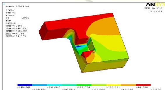
Fig – 3.14 : Stress in Y- Direction
