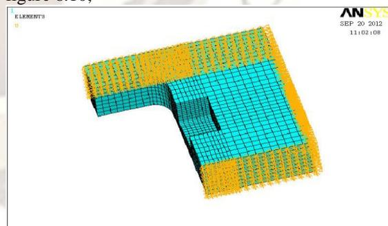
FIG – 3.10 : Submodel along with the boundary conditions
