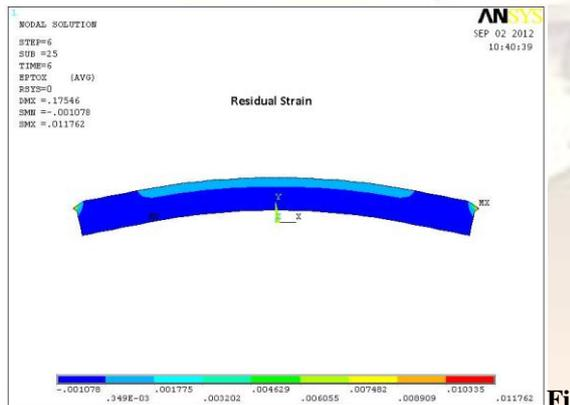
Fig – 2.8: At load 0N Residual strain
