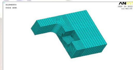
Fig – 3.9: Submodel of the selected region with the mesh.
