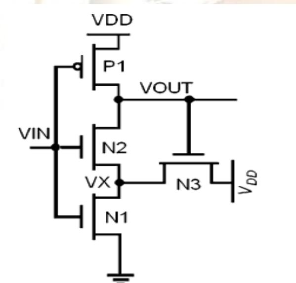
Figure 2: Modified Schmitt- trigger used to form the inverter of memory bitcell.
