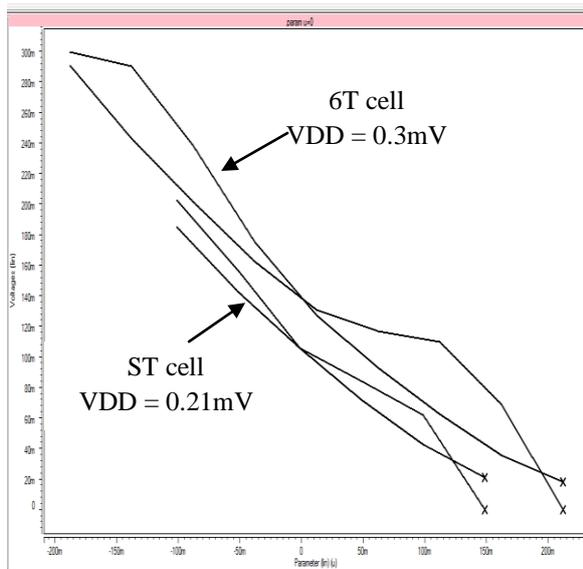
Figure 5: Read SNM failure comparison of 6T bitcell and ST based bitcell at lower supply voltage (VDD=400mV)
