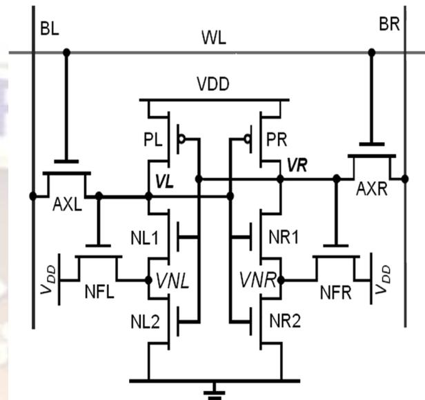
Figure 3: schematic for the ST based SRAM bitcell
