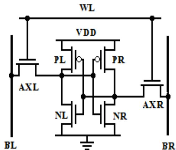
Figure 1: 6T SRAM cell
