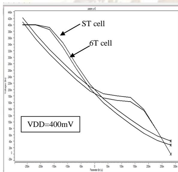
Figure 4: Read SNM curve for 6T and ST based bitcell at lower supply voltage (VDD=400mV)
