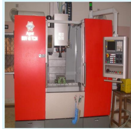
Fig.3. 1 : CNC Milling Machine – Vertical Machining Centre
