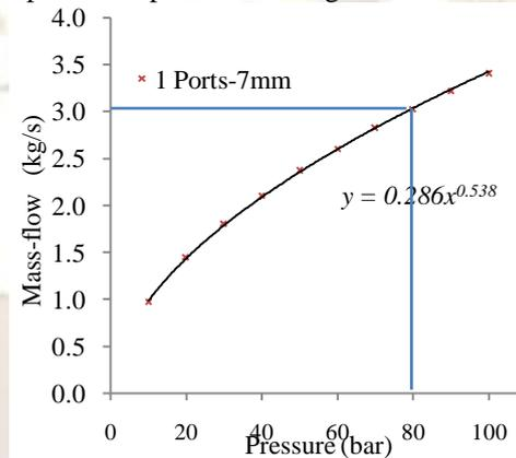
Figure 5: mass rate vs. load pressure.
