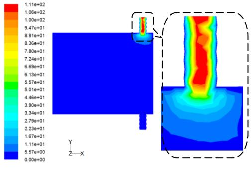
Figure 3: velocity contours for single outlet port.
