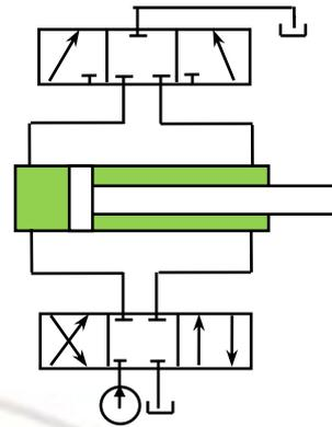
Figure 8: the proposed hydraulic circuit. The inlet flow to the cylinder in the proposed system remains as it was in the conventional cylinder.
