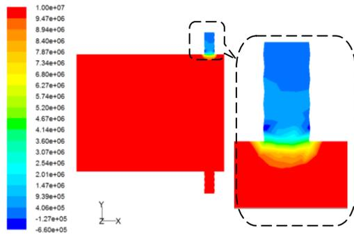
Figure 2: static pressure contours for single outlet port.
