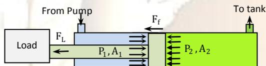
Figure 1: a loaded cylinder actuator.
