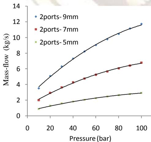
Figure 11: mass rate vs. load pressure.
