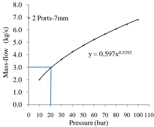
Figure 10: mass rate vs. outlet port size.
