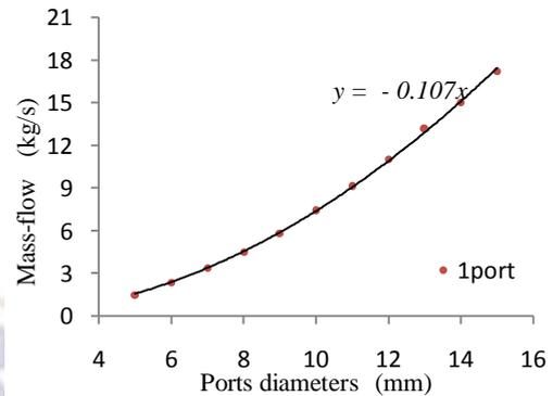
Figure 4: mass rate vs. ports diameters
