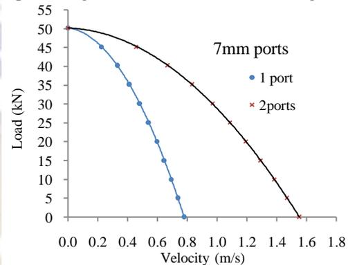
Figure 12: load vs. velocity in hydraulic cylinder.
