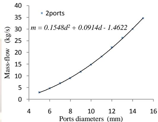
Figure 9: mass rate vs. ports diameters.
