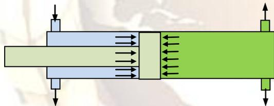
Figure 7: the proposed four ports hydraulic cylinder actuator.
