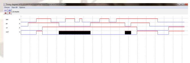
Fig3b: Simulation results of Ultra Low-power 8T SRAM Cell
