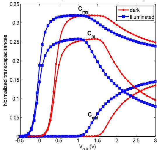
Fig 9 Normalized transcapacitances with  $V_{DS}=1V$ , varying  $V_{GS}$  under dark and with optical flux of  $1 \times 10^{14}$
