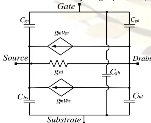
Fig. 3 Small Signal model for low and medium frequency
