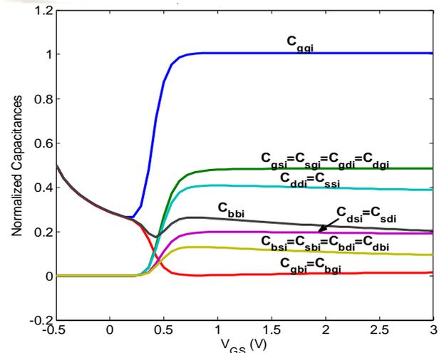
Fig 5 Intrinsic Capacitances under dark condition at  $V_{DS}=0V$  and varying  $V_{GS}$ .
