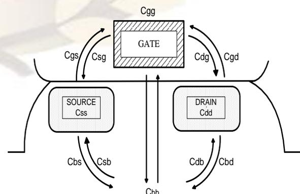
Fig. 2 Intrinsic Capacitances in MOSFET
