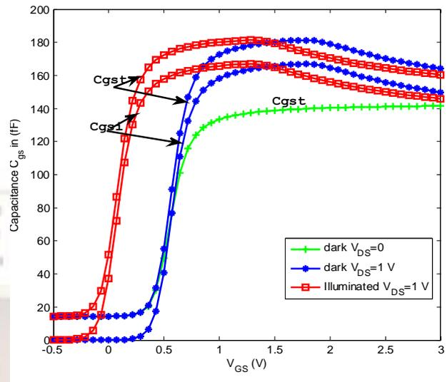
Fig 11 Capacitance  $C_{gst}$  and  $C_{gsi}$  under dark and Illumination.
