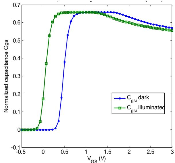
Fig 8 Intrinsic Capacitance  $C_{gsi}$  with  $V_{DS}=1V$ , varying  $V_{GS}$  under dark and with optical flux of  $1 \times 10^{14}$ .
