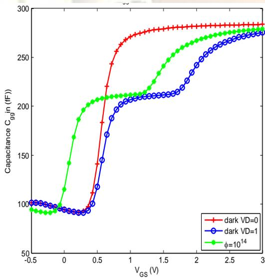
Fig 10 Total Capacitance  $C_{gg}$  with varying  $V_{GS}$  and  $V_{DS}$  under dark and with optical flux of  $1 \times 10^{14}$ .
