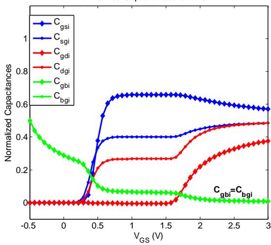
Fig 7 Additional Intrinsic Capacitances Components with  $V_{DS}=1V$  and varying  $V_{GS}$  under dark condition.
