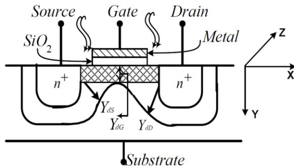
Fig. 1 Schematic of MOSGET under illumination
