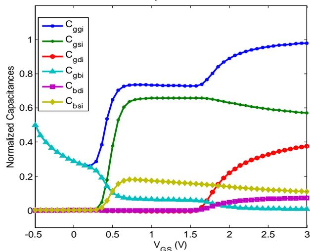
Fig 6 Significant Intrinsic Capacitances with  $V_{DS}=1V$  and varying  $V_{GS}$  under dark condition.
