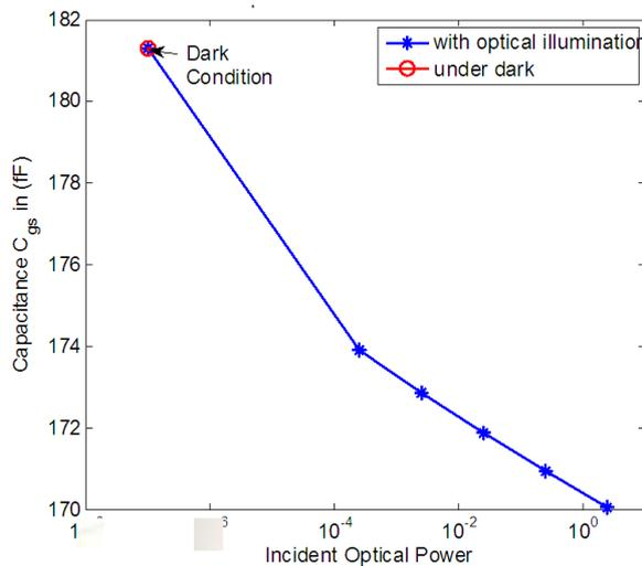
Fig 13 Capacitance  $C_{gst}$  under dark and with varying optical flux of  $1 \times 10^{14}$  to  $1 \times 10^{18}$
