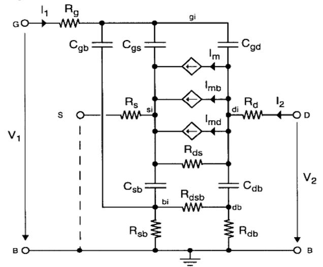
Fig.4 Small Signal model valid at RF.
