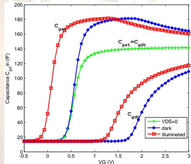
Fig 12 Total capacitances  $C_{gst}$  and  $C_{gdt}$  under dark and illumination.
