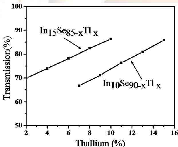
Figure 3: The variation of percentage of transmittance with thallium content of In<sub>10</sub>Se<sub>90-x</sub>Tl<sub>x</sub> and In<sub>15</sub>Se<sub>85-x</sub>Tl<sub>x</sub> glassy systems.
