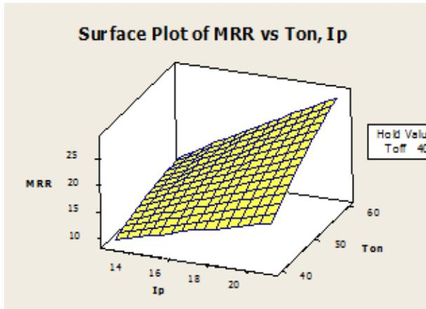
Figure 1: Effect of Ip & Ton on MRR
