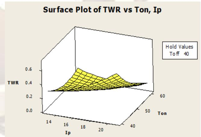
Figure 4: Effect of Ip & Ton on TWR
