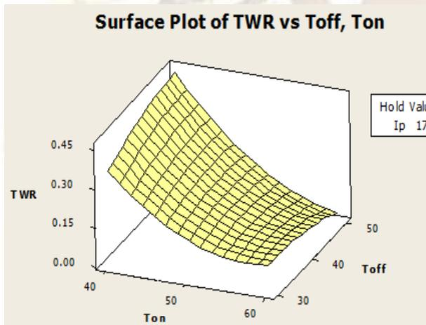
Figure 6: Effect of Ton & Toff on TWR
