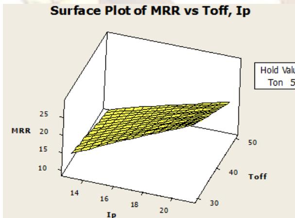
Figure 2: Effect of Ip & Toff on MRR
