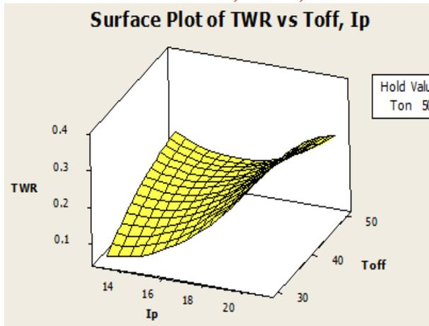
Figure 5: Effect of Ip & Toff on TWR
