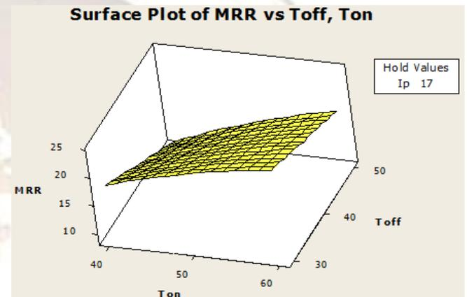
Figure 3: Effect of Ton & Toff on MRR
