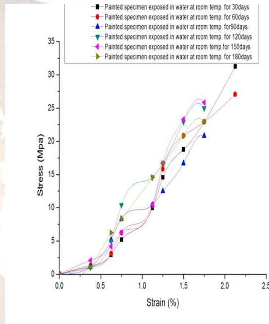
Graph 2: Tensile test -Stress-Strain for painted specimen exposed in water at room temperature (Specimen exposure time 30days to 180days)
