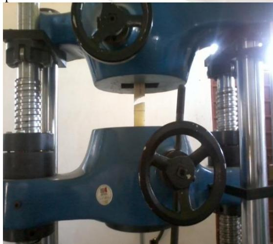
Fig.6 Tensile testing on UTM
