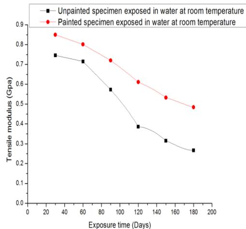
Graph 6: Tensile Stress V/S Exposure time for unpainted and painted specimen exposed in water at room temperature (Specimen exposure time 30 days to 180 days)
