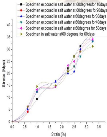
Graph.5: Tensile test -Stress-Strain unpainted specimen exposed in salt water at constant temperature 60°C (Specimen exposure time 10 days to 60 days)
