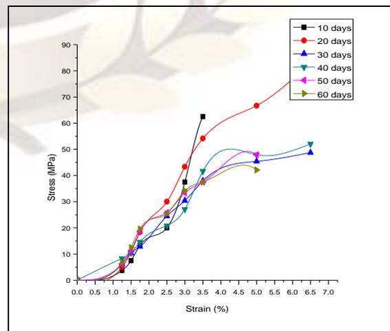
Graph.3: Tensile test -Stress-Strain unpainted
