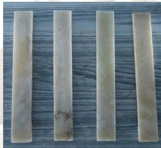
Fig.3. Test specimens produced from laminate
