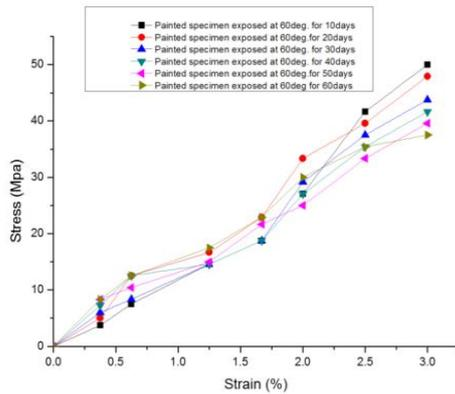
Graph.4: Tensile test -Stress-Strain painted specimen exposed in water at constant temperature 60°C (Specimen exposure time 10 days to 60 days)
