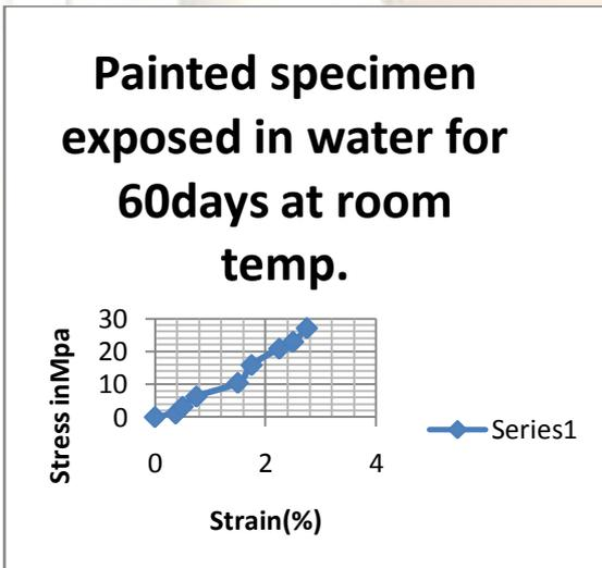
Tensile modulus painted specimen (60 Days),  $E_2 = (7.0/0.8+7.80/1+12/1.2)/3*100 \text{ N/mm}^2$
