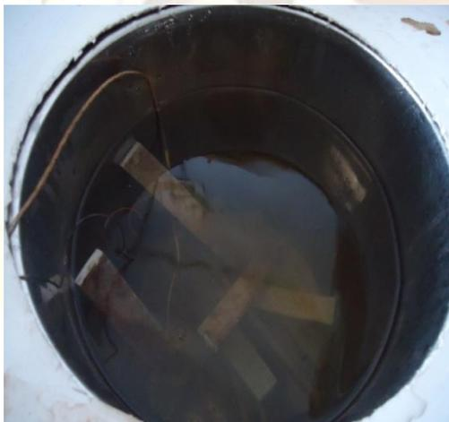
Fig.5. Constant temperature water bath with specimens
