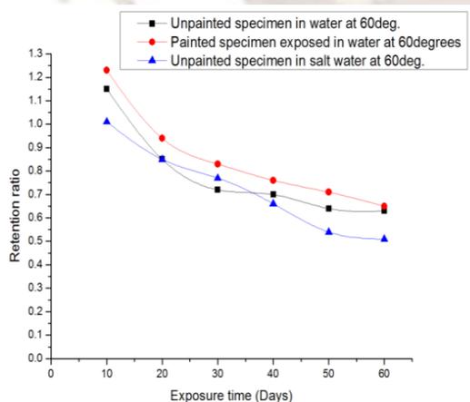
Graph9: Retention ratio V/S Exposure time for unpainted and painted specimen exposed in water and salt water at 60°C temperature (Specimen exposure time 10days to 60days).
