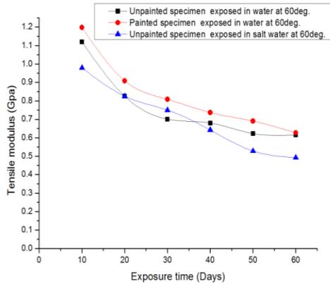
Graph7: Tensile Stress V/S Exposure time for unpainted and painted specimen exposed in water and salt water at 60°C temperature (Specimen exposure time 10days to 60days).
