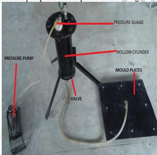
Fig. 1: RTM (Resin transfer molding )Machine
