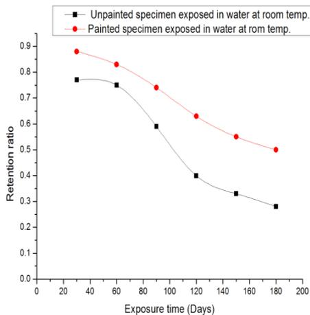
Graph.8:Retention ratio V/S Exposure time for unpainted and painted specimen exposed in water at room temperature (Specimen exposure time 30days to 180days)
