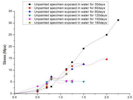
Graph.1: Tensile test -Stress-Strain for unpainted specimen exposed in water at room temperature (Specimen exposure time 30days to 180days)
