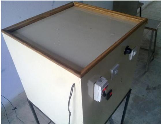
Fig.4 Constant temperature water bath
