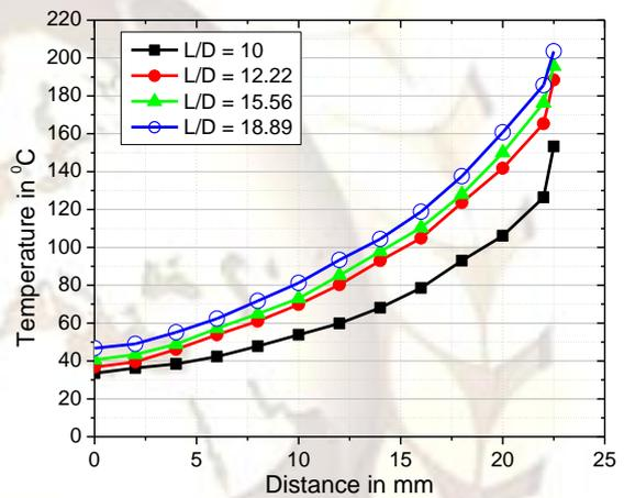
Fig. 6. Temperature profiles at the channel exit for smooth tubes with different length
