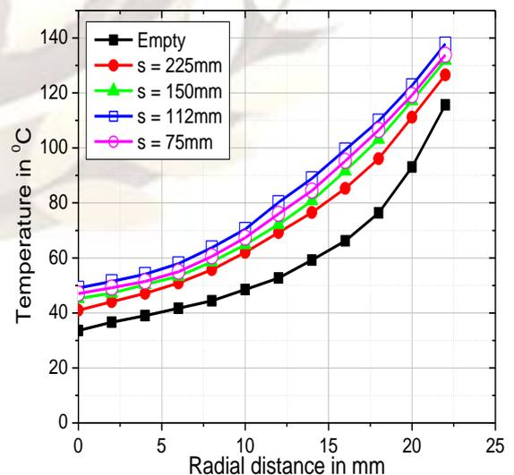
Fig. 7. Temperature profiles at the channel exit for tubes with discrete rings
