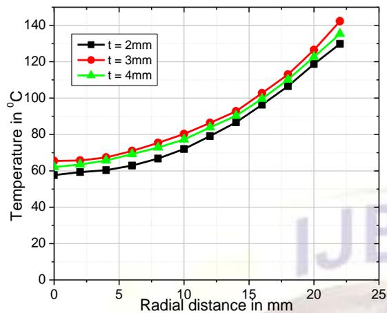
Fig. 8. Temperature profiles at the channel exit for different ring spacing
