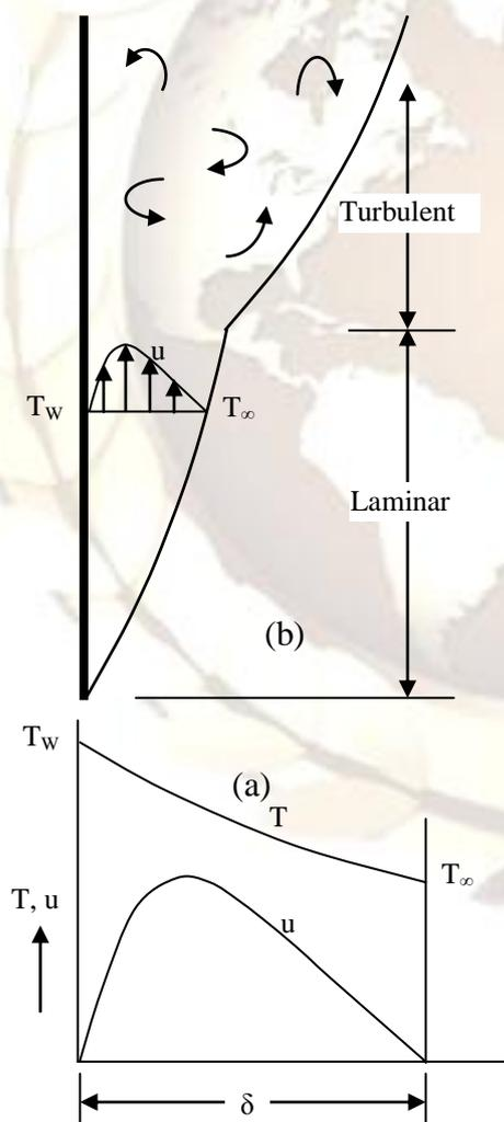
Fig. 1.(a) Boundary layer on a vertical flat plate (b) Velocity and Temperature distribution in the boundary layer
