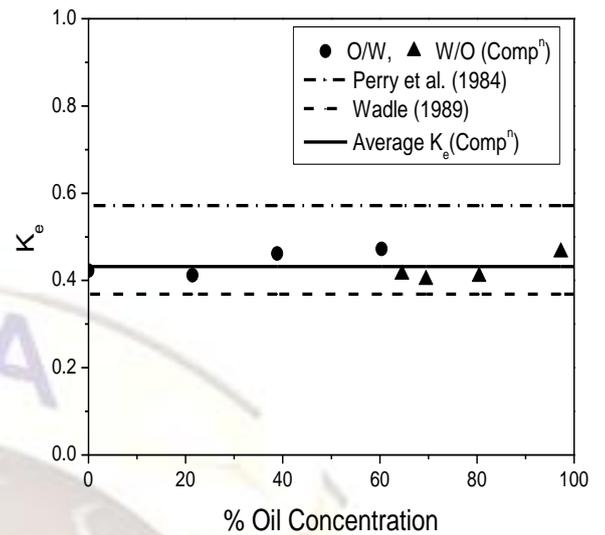
Fig.8. Expansion loss coefficient as a function of oil concentration
