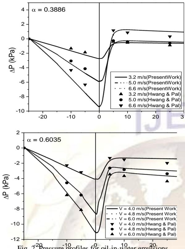
Fig. 2. Pressure profiles for oil-in-water emulsions flowing through a sudden expansion
