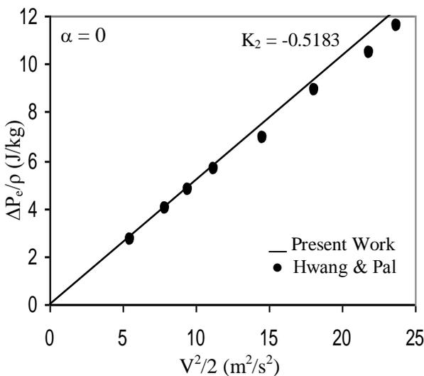
Fig. 6.  $\Delta P_e/\rho$  versus  $V^2/2$  for oil-in-water emulsions flowing through a sudden expansion
