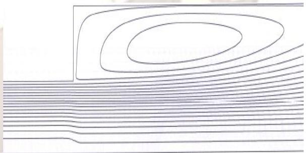
Fig. 4. Stream lines for  $\alpha = 0.2144$  and  $v = 6.8$  m/s
