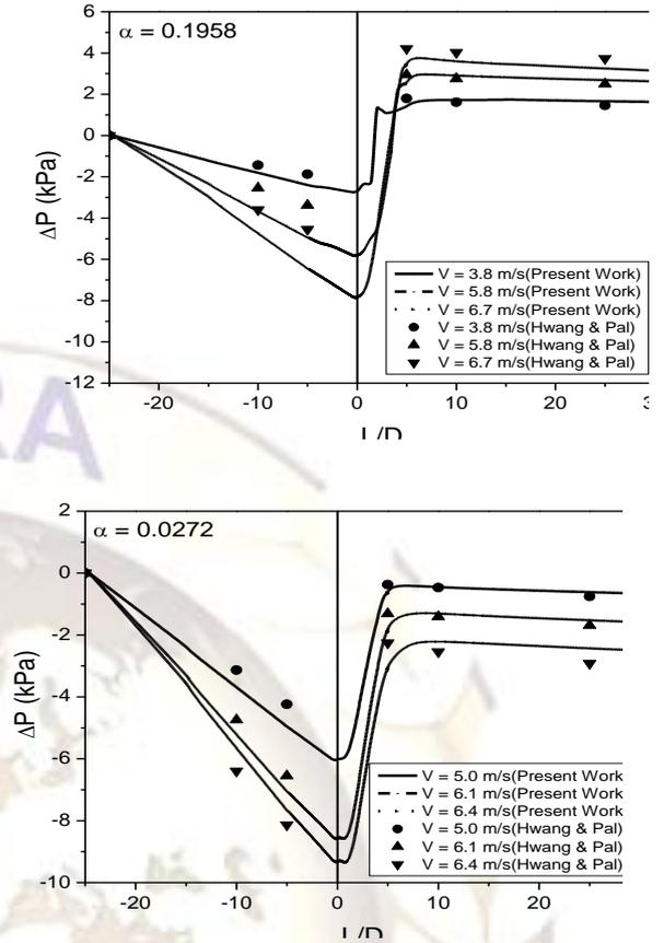
Fig. 3. Pressure profiles for water-in-oil emulsions flowing through a sudden expansion
