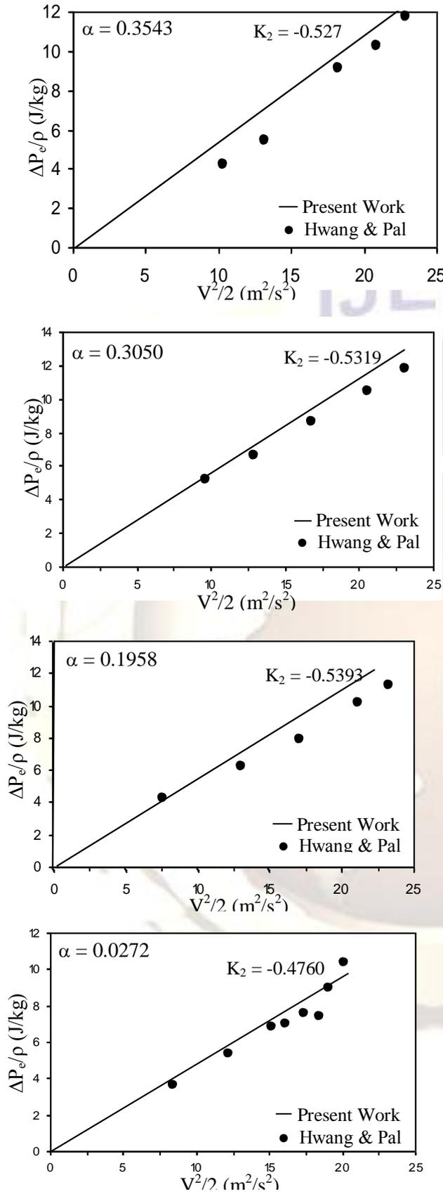
Fig.7.  $\Delta P_e/\rho$  versus  $V^2/2$  data for water-in-oil emulsions flowing through a sudden expansion
