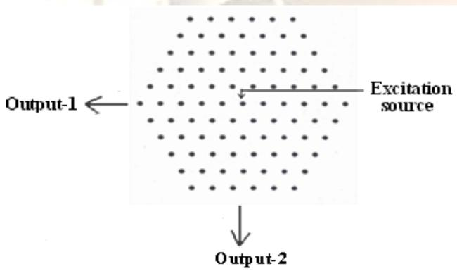
Figure 1. Hexagonal structure of PCFs
