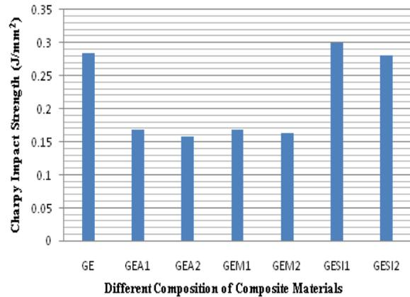
Fig. 6 Charpy Impact strength for different composition of composite materials
