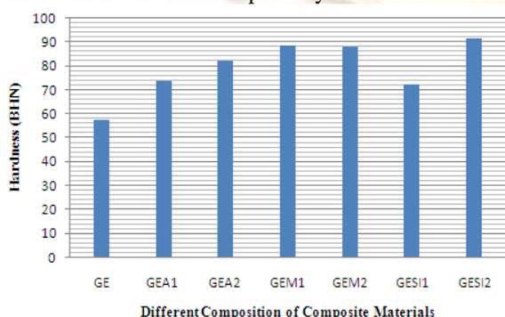
Fig. 8 Brinell hardness number for different composition of composite materials
