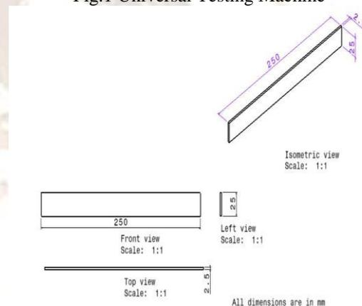
Fig. 2 Tensile strength test specimen
