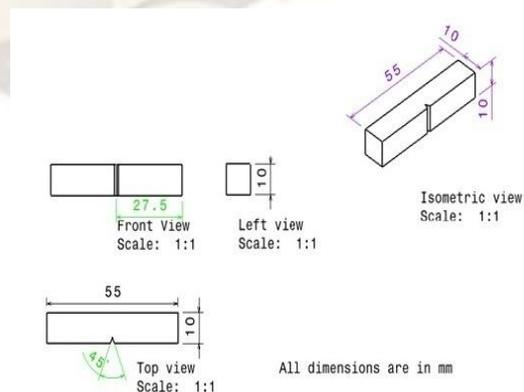
Fig. 3 Charpy Impact Test Specimen
