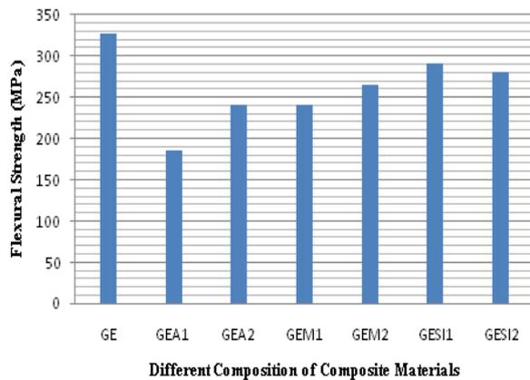
Fig. 7 Flexural strength for different composition of composite materials
