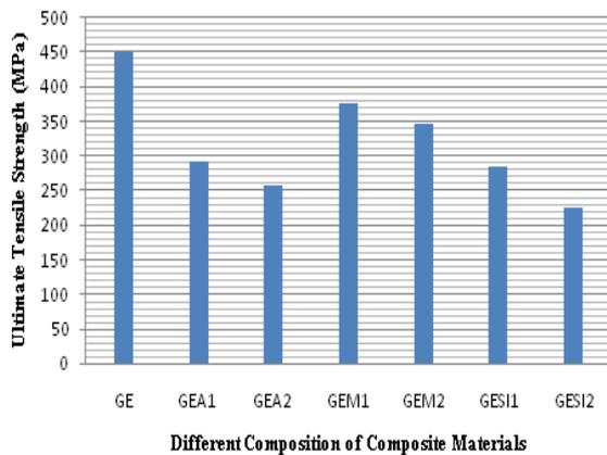
Fig.5 Ultimate tensile strength for different composition of composite materials
