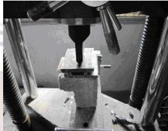
Fig. 8 L-Type Specimen under Shear
