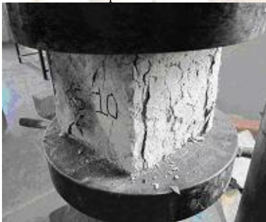
Fig. 2 RS10 Cube under Compression
