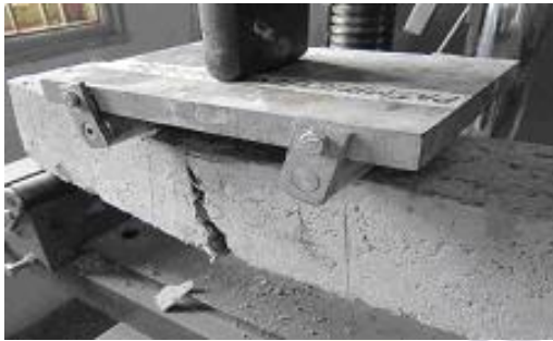
Fig. 5 Beam Testing for Flexural Strength
