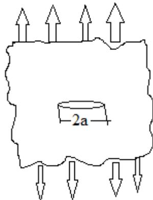
**A) Infinite Plate With Centre Through Crack Under Tension**
