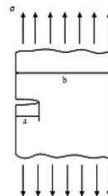
**d) Infinite stripe with an edge through crack under tension**
