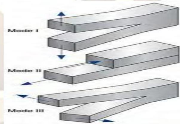
**Figure 1: Three Types Of Loading On A Cracked Body;**
