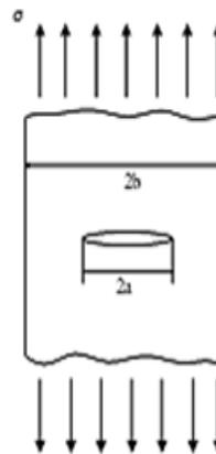
**c) Infinite stripe with a centre through crack under tension**
