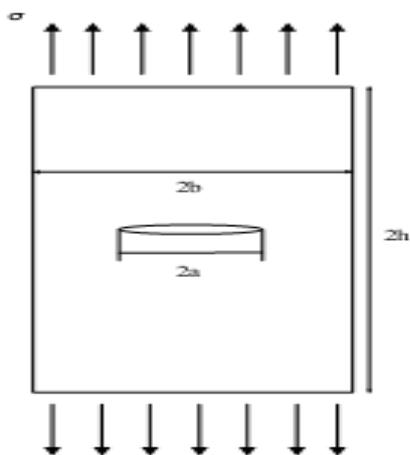
**FIGURE. 4: Finite Plates With A Centre Through Crack Under Tension**
