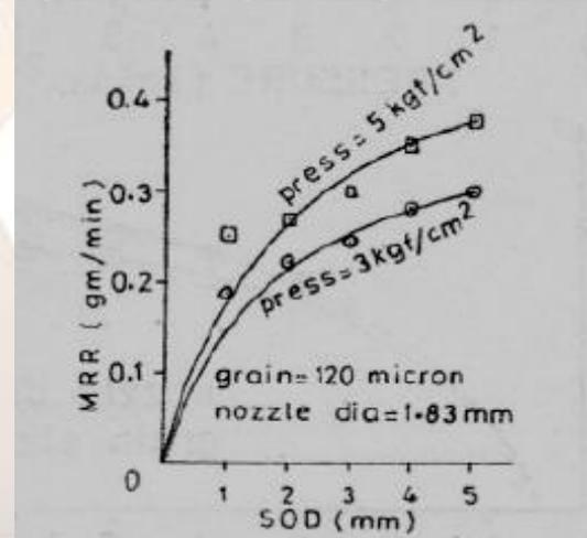
Figure 2: MRR vs SOD
