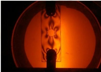
Fig.15. Isochromatic Fringe pattern for circular cutout.
