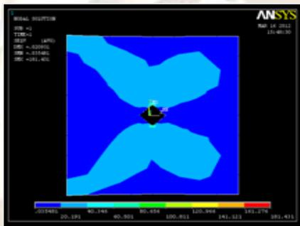
Fig.13. Stress contour for square cutout ( $r/R = 0.1$ ,  $\theta = 45^\circ$ )
