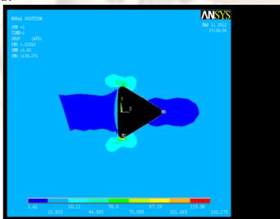
Fig 8. Von-misses Stress contour for plate with triangular cutout ( $r/R = 0.1$ )
