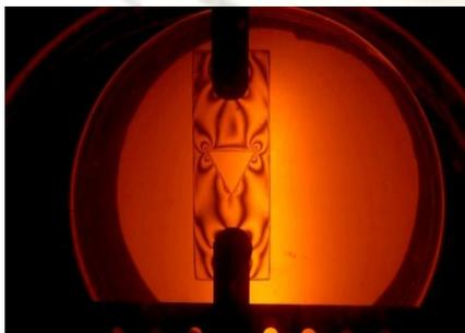
Fig.17. Isochromatic Fringe pattern for triangular cutout.
