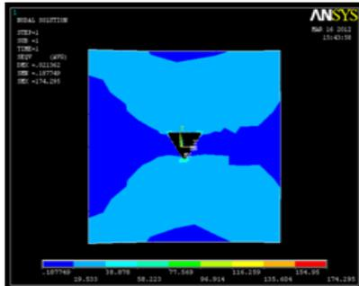
Fig.12. Stress contour for triangular cutout ( $r/R = 0.1$ ,  $\theta = 30^\circ$ )
