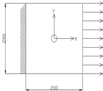
Fig.1 Loading condition ; Axial tensile pressure (all dimensions in mm)
