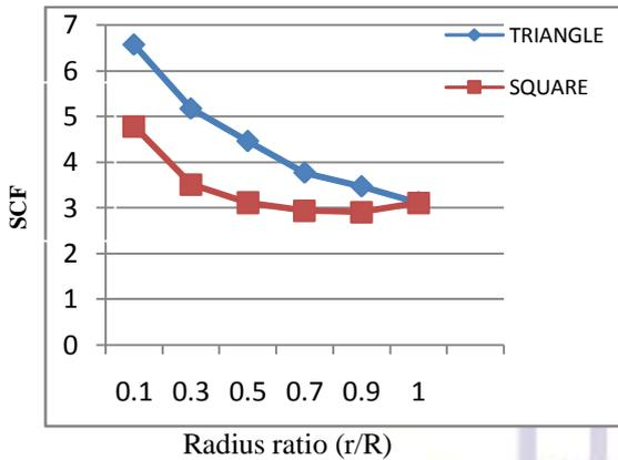
Fig 7. SCF with respect to radius ratio
