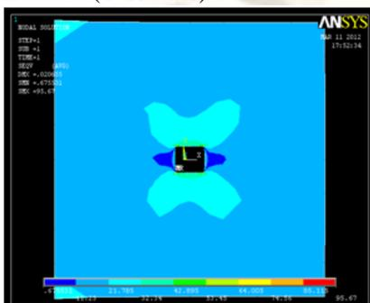
Fig.9.Von- Misses Stress contour for plate with square cutout ( $r/R = 0.1$ )
