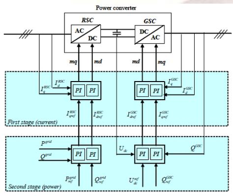
Fig.2. Control structure of DFIG
