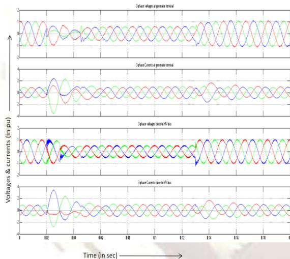
Fig.5 Voltages and currents at generator terminal and MV bus for a 3-phase fault at generator terminal
