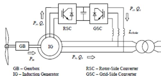
Fig.1. DFIG connected to a grid
