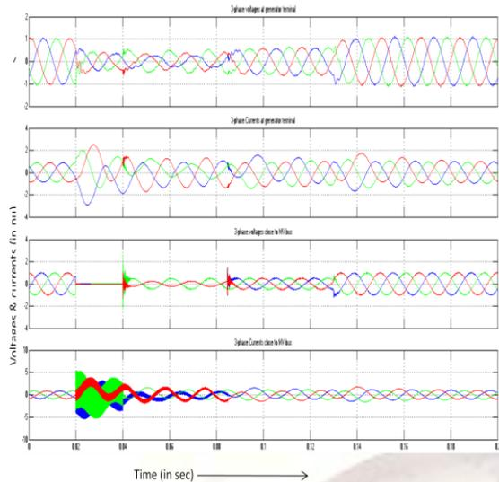
Fig. 4. Voltages and currents at generator terminal and MV bus for a 3-phase fault at MV Bus
