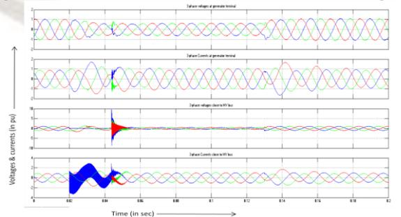
Fig.8 Voltages and currents at generator terminal and MV bus for a Phase-ground fault at MV Bus
