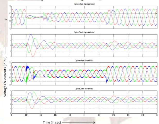
Fig. 3 Voltages and currents at generator terminal and MV bus for a 3-phase fault at generator terminal Voltage drop on the MV bus is marginal when compared to the voltage drop at the generator terminal. This is due to the positive sequence generator step-up transformer impedance, positive sequence impedance of the collector cable section and the fault resistance.
