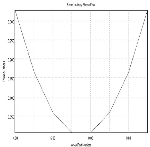
Fig.4 Phase distribution of Rotman Lens.
