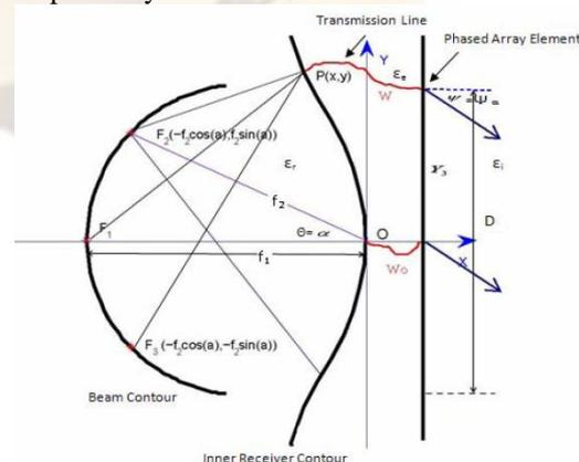
Fig.1 Trifocal Rotman Lens Schematic Diagram.
