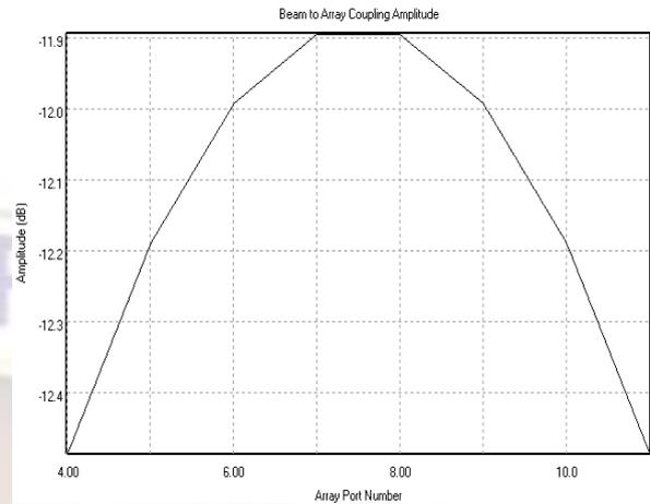
Fig.5 Amplitude distribution of array ports.
