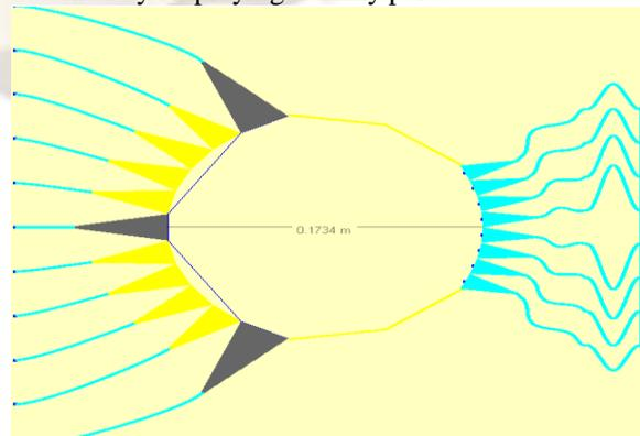
Fig.2 Simulated Rotman Lens.
