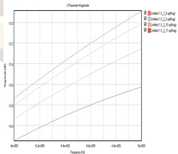
Fig.7 S-parameter(S2\_8 to S2\_11) magnitude vs. frequency.
