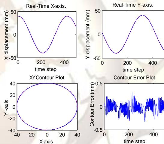
Fig. 13 Experimental result using 15<sup>th</sup> order filter for minimum phase model
