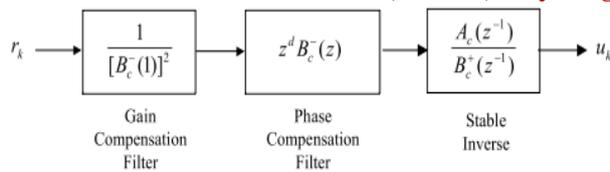
Fig.6 ZPETC structure block diagram
