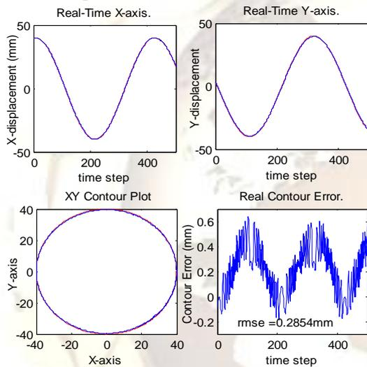
Fig. 11 Experimental results using ZPETC for minimum phase model
