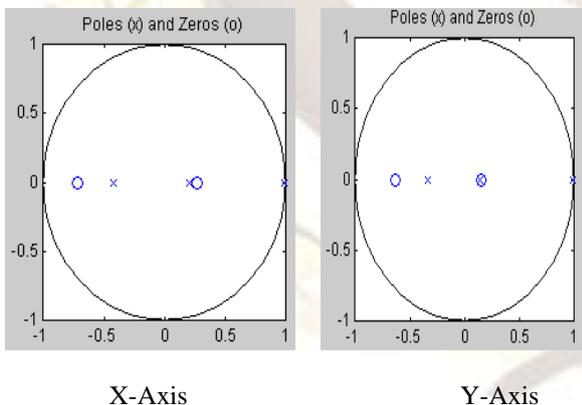
Fig.4 Zero-pole plot for x and y axis for 60ms sampling time
