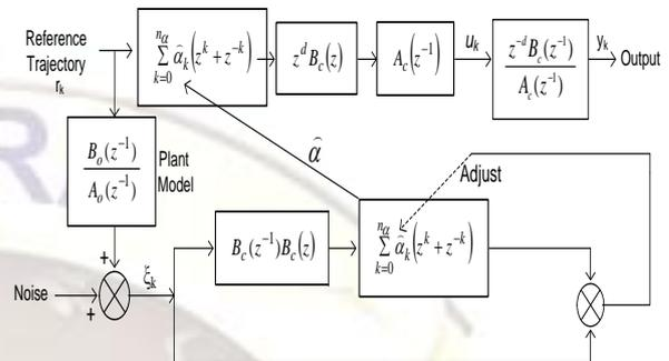
Fig. 9 Feedforward ZPETC without factorization of zeros
