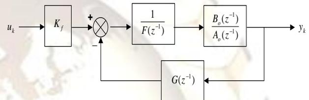
Fig. 6 Pole placement feedback control system block diagram
