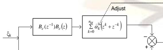
Fig. 8 Adaptive ZPETC gain filter
