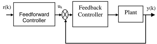
Fig.5 Control system block diagram
