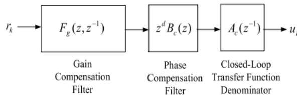
Fig. 7 ZPETC without factorization of zeros polynomial
