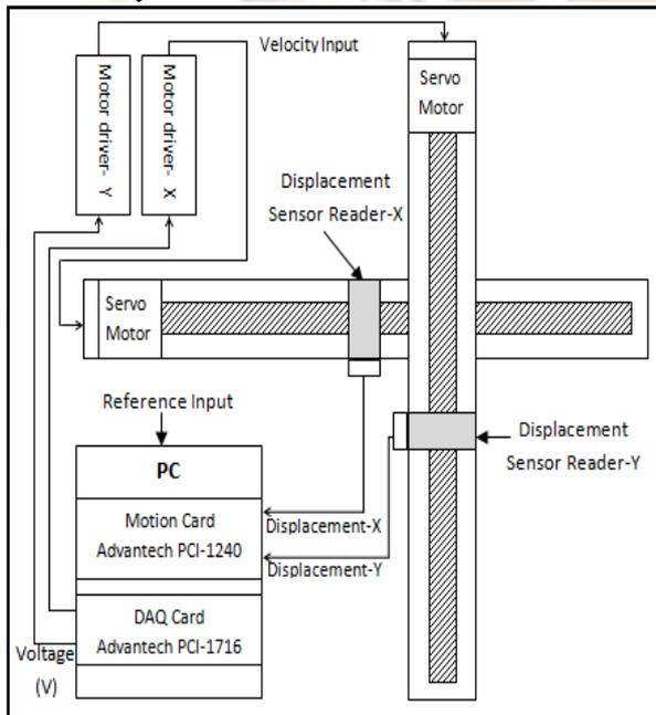
Fig. 1 Plant schematic diagram
