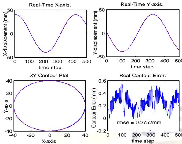
Fig. 10 Experimental results using ZPETC for non-minimum phase model
