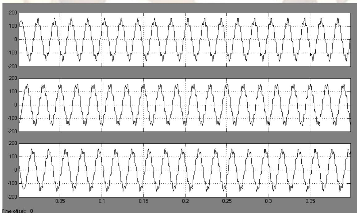
Fig.7 Source voltage containing harmonics
