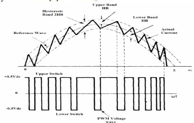
Fig.5 Basic principle of hysteresis band control
