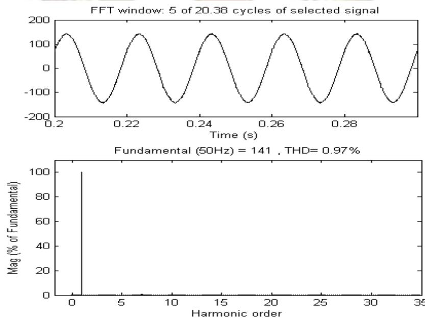
Fig.11 FFT Analysis for load voltage
