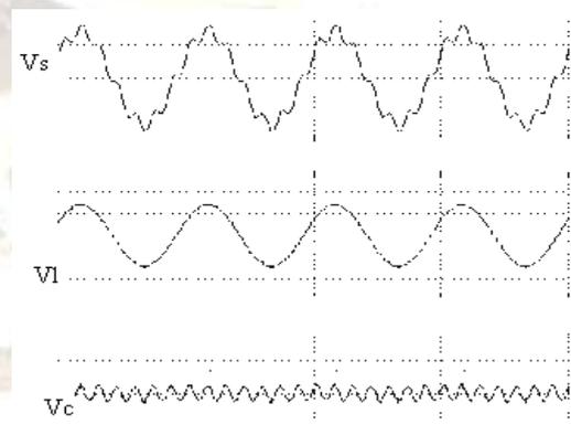
Fig.3 Waveforms for the supply voltage ( $V_s$ ), Desired load voltage ( $V_l$ ) and the Compensating voltage (filter voltage- $V_c$ )
