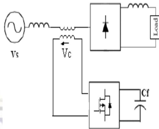
Fig.2 Basic compensation principle
