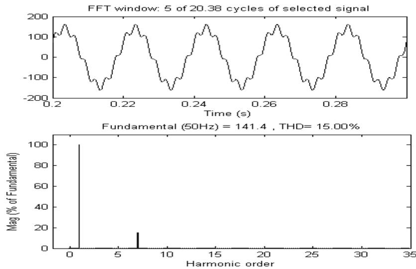
Fig.10 FFT Analysis for source voltage
