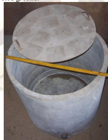
Fig 3 Ferro-cement cylindrical test mould
