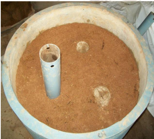
Fig.6b Removal of casing for the third vertical drain
