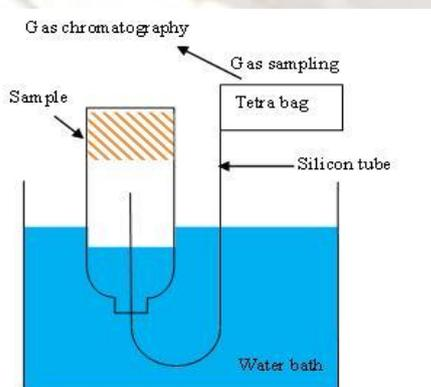
Fig 5. Schematic of gas chromatography measuring device.
