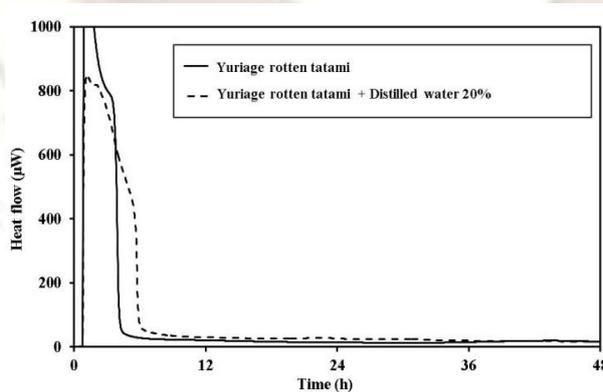
Fig 10. TAM results of Yuriage rotten tatami (untreated samples)
