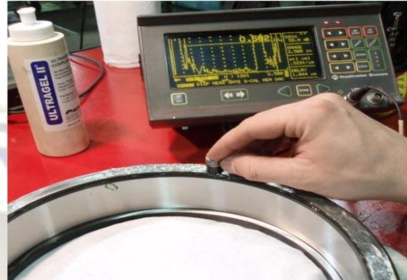
Figure 6: Ultrasonic Flaw Detector
