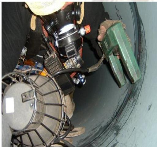
Figure 5: Magnetic Particle Testing
