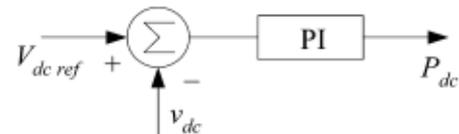
Fig. 2. Schematic diagram of the conventional dc-link voltage controller.
