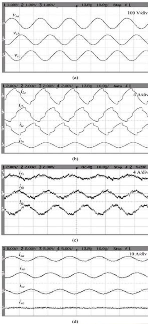
Fig.8(a)Supply voltages.(b)Load currents.(c)
