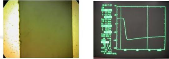
(c) Micro-channel image after etching time of 60 min.(etched depth: 29.82  $\mu\text{m}$ )
