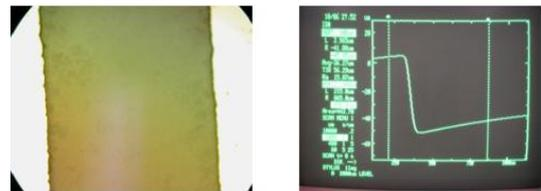
(b) Micro-channel image after etching time of 10 min.(etched depth: 4.97  $\mu\text{m}$ )
