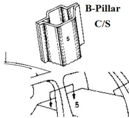
**Fig. 2 B-Pillar C/S of B-pillar of a passenger car**
