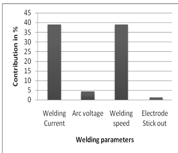
Fig.3 : Influence of process parameters on bead penetration.
