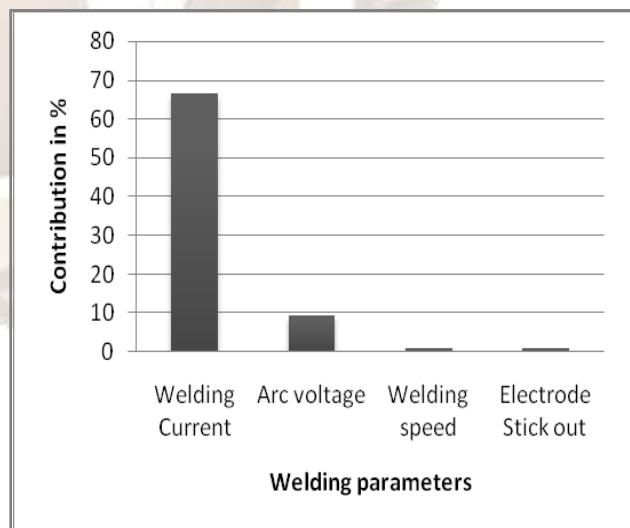
Fig.2: Influence of process parameters on bead width.
