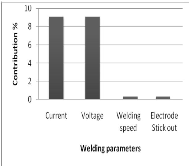
Fig.4: Influence of process parameters on weld reinforcement.
