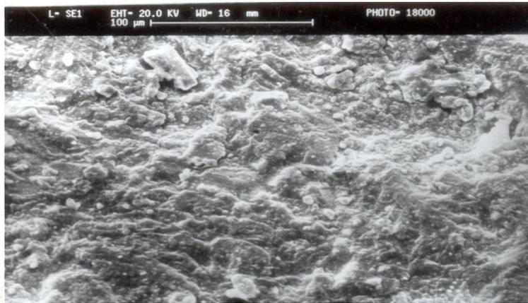
Fig. 17 Scanning electron micrograph of the vacuum sintered Al-10 weight % SiC<sub>p</sub> composite sample at magnification 360X
