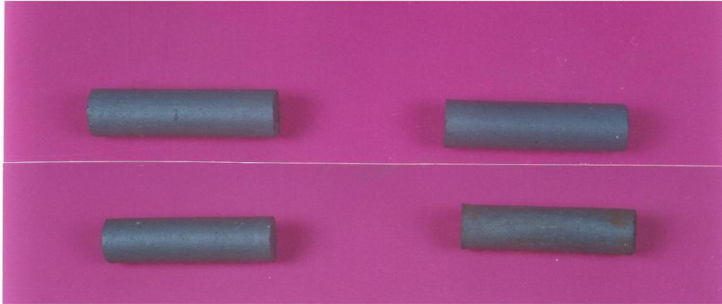
Fig. 4 Photograph of the Al-SiC<sub>p</sub> composite specimens fabricated by powder metallurgy process.
