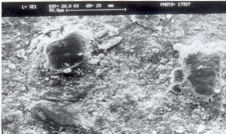
Fig. 18 Scanning electron micrograph of the vacuum sintered Al-20 weight % SiC<sub>p</sub> composite sample at magnification 600X
