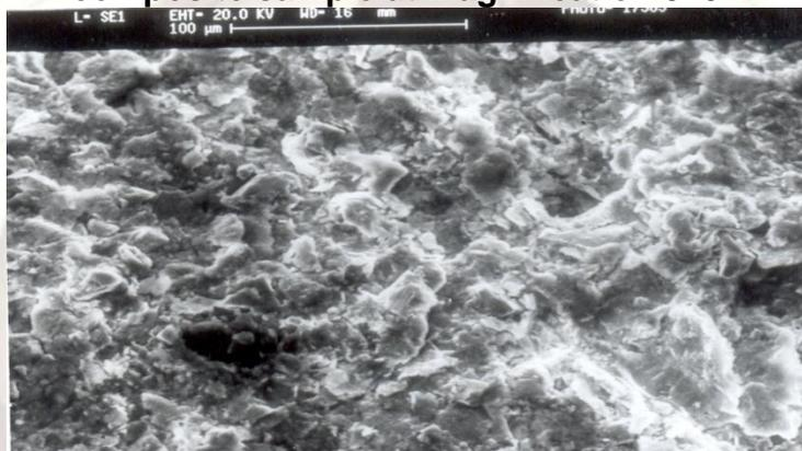
**Fig. 15 Scanning electron micrograph of un-sintered Al-20 weight % SiC<sub>p</sub> composite sample at magnification 340X**
