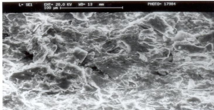
**Fig. 14 Scanning electron micrograph of un-sintered Al-10 weight % SiC<sub>p</sub> composite sample at magnification 340X**
