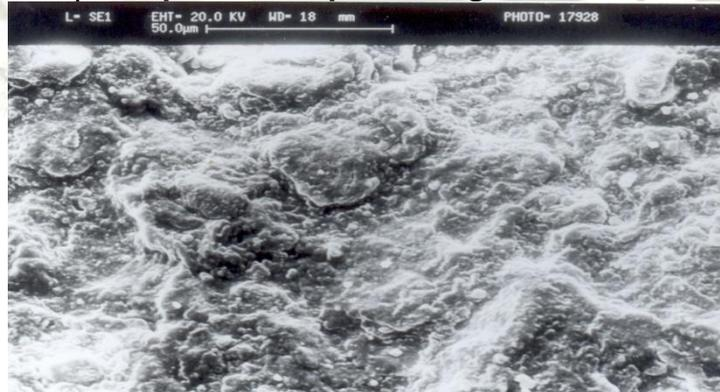
Fig. 19 Scanning electron micrograph of the vacuum sintered Al-30 weight % SiC<sub>p</sub> composite sample at magnification 600X.
