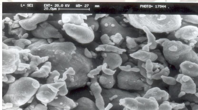
**Fig. 3 Scanning electron micrograph of SiC particulates used in the present work**
