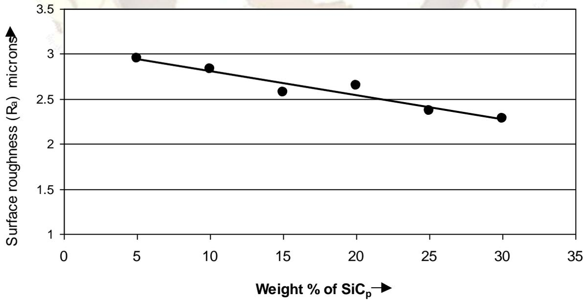
Fig. 13 Surface roughness of PM Al-SiC<sub>p</sub> composites
