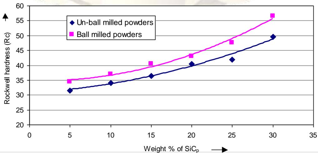
Fig. 7 Rockwell hardness of isostatically pressed Al-SiC<sub>p</sub> composites prepared using un-ball milled and ball milled powders 431 | Page
