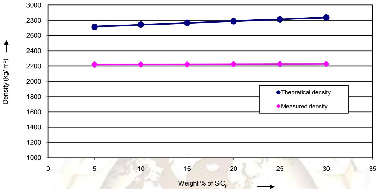
Fig. 9 Density of sintered Al-SiC<sub>p</sub> composites
