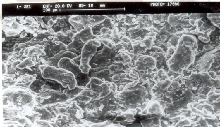
**Fig. 16 Scanning electron micrograph of un-sintered Al-30 weight % SiC<sub>p</sub> composite sample at magnification 340X**
