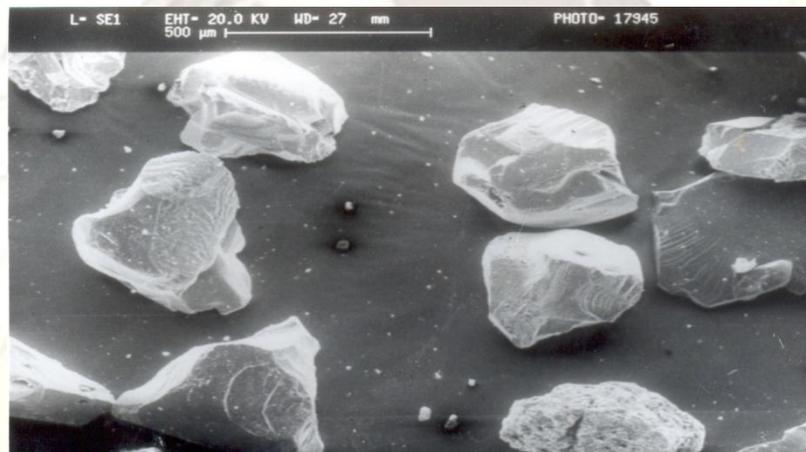
**Fig. 2 Scanning electron micrograph of the aluminum powders used in the present work**
