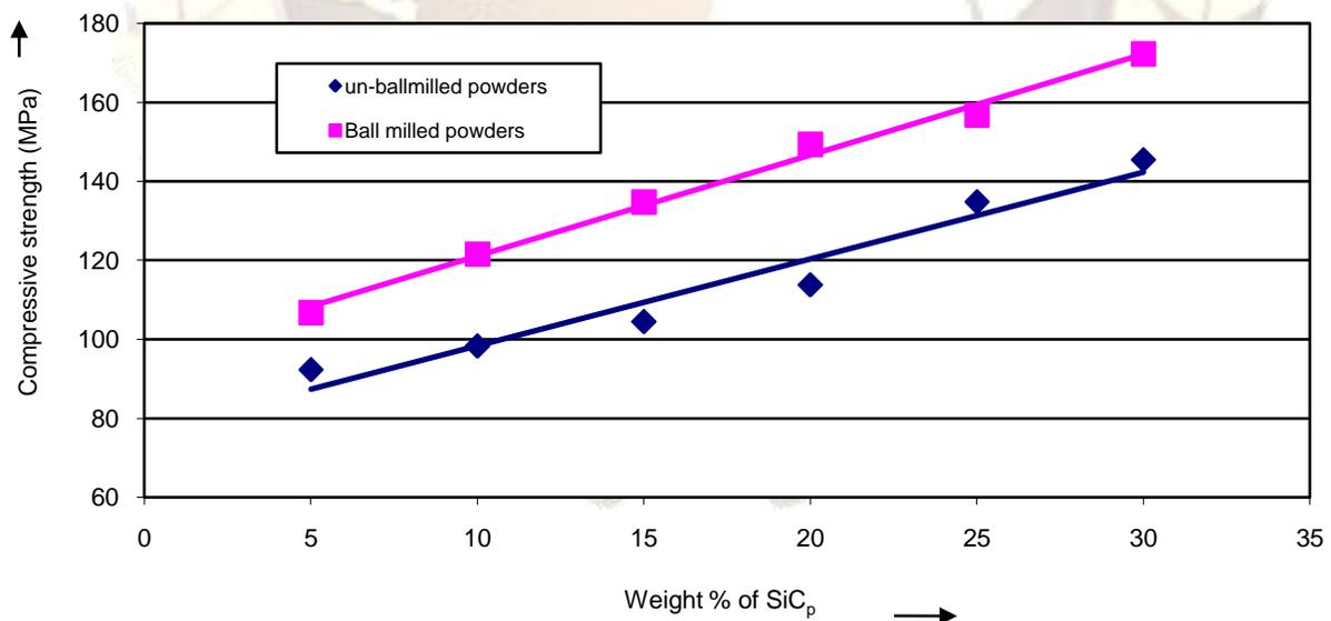
Fig. 11 Compressive strength of sintered Al-SiC<sub>p</sub> composite samples prepared from un-ballmilled and ballmilled powders
