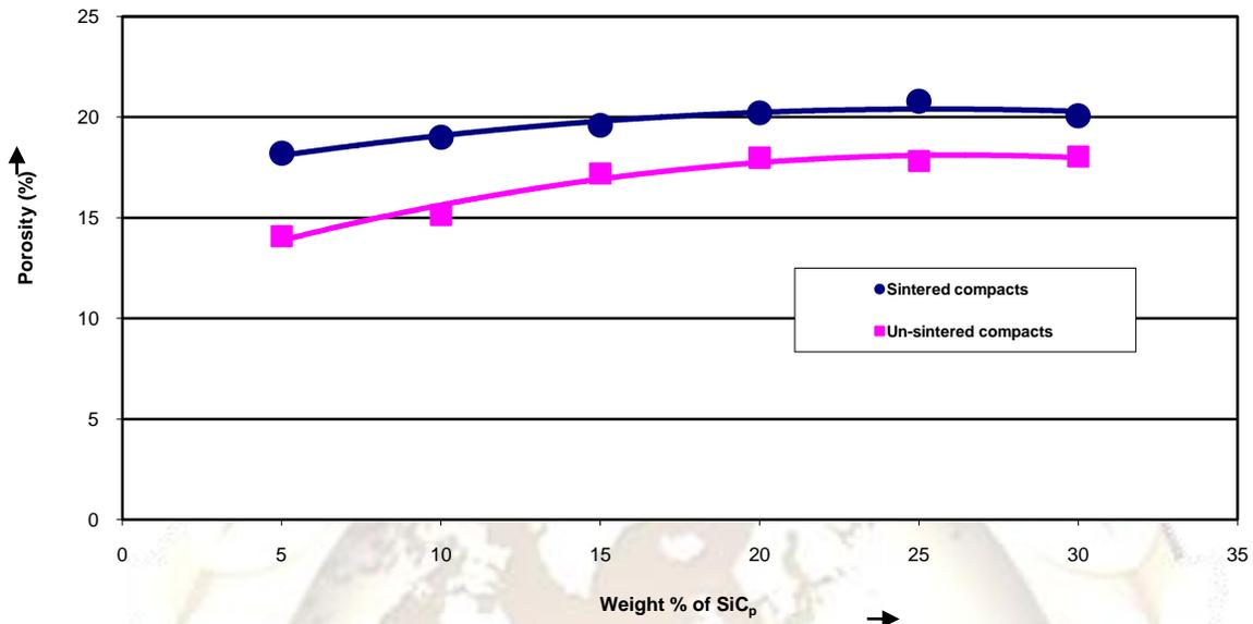
Fig. 10 Porosity of Al-SiC<sub>p</sub> composites in green and sintered conditions
