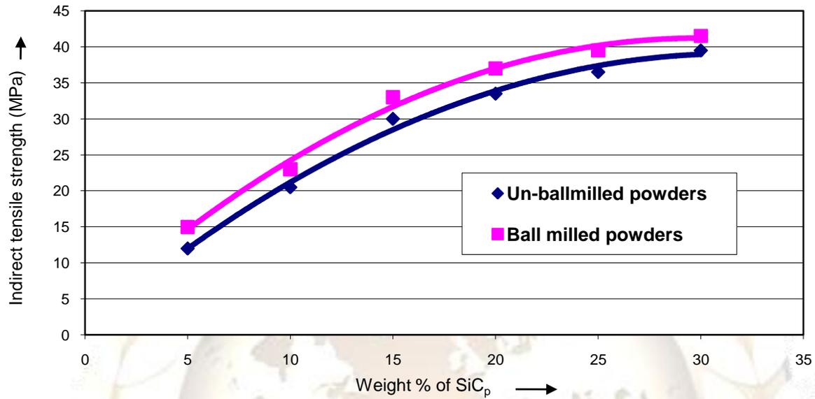
Fig. 12 Indirect tensile strength of PM Al-SiC<sub>p</sub> composite fabricated using un-ballmilled and ballmilled powders
