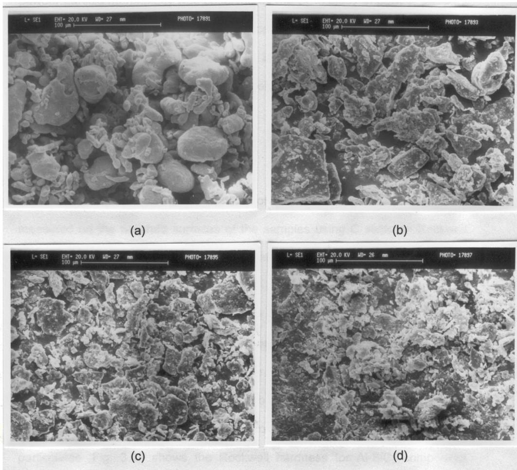
Fig. 6 Scanning electron micrographs of the Al powders with 30 weight % of SiC particulates (a) before ball milling, irregular particles; (b) after 4 hours of ball milling, flat lamellaer structure; (c) after 8 hours of ball milling, cluster type structure and (d) after 12 hours of ball milling, equiaxed. (Mag. X400)
