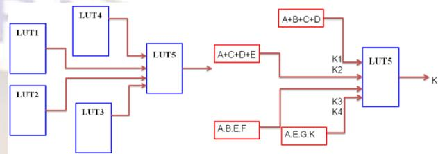
Figure 6. Master LUT- Predecessor architecture and detailed diagram for the functionality of Predecessors
