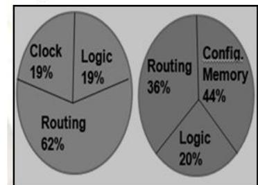
Figure2. Breakdown of dynamic & Static power consumption in Xilinx Spartan-3 FPGAs
