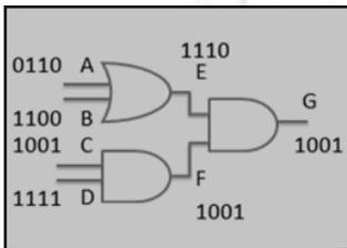
Figure 3. Propagation of simulation vectors
