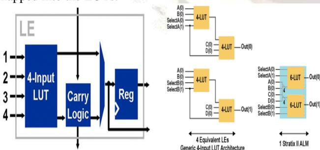
Figure 5. 4-input Logic Element(LE) block diagram (Altera's Stratix FPGA family).
