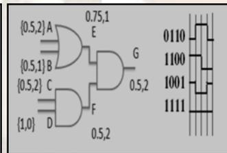
Figure 4. Propagation of statistical parameters
