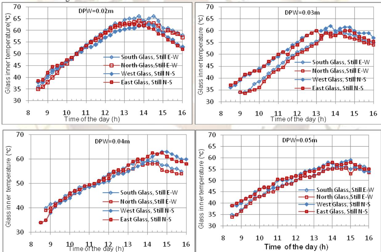
Fig.4.1 Variation in glass inner surface temperature for different depths and orientation
