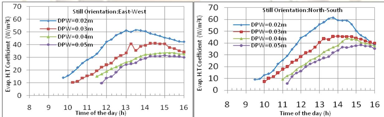
**Fig.4.3. Variation in evaporative heat transfer coefficient**
