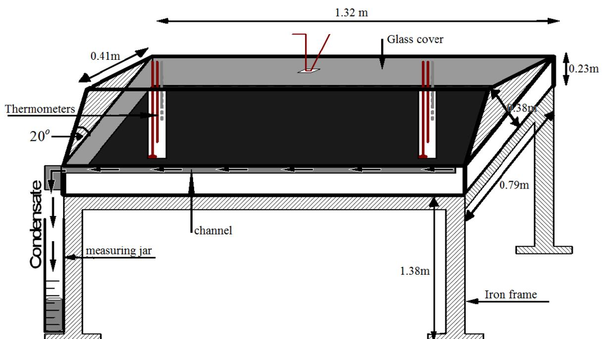
Fig. 2.1 Schematic diagram showing dimensions of the still
