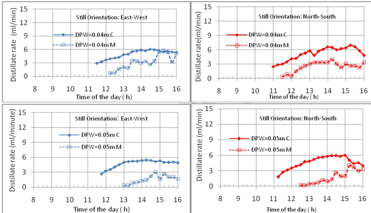
Fig.4.5. Comparison of calculated and measured distillate output
