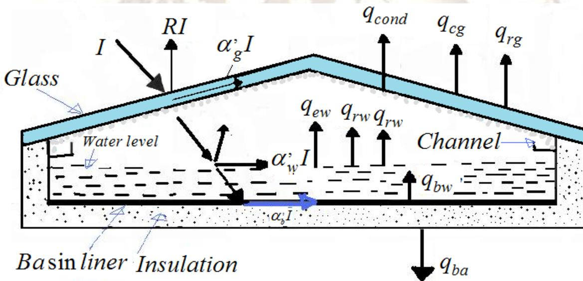
Fig.3.1 Cross sectional view of a double slope solar still
