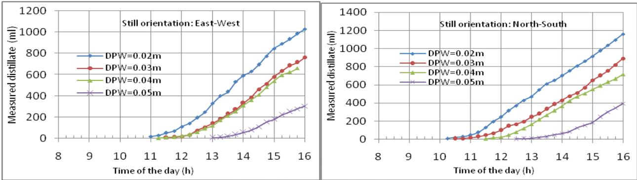
Fig.4.4. Variation in the measured distillate output
