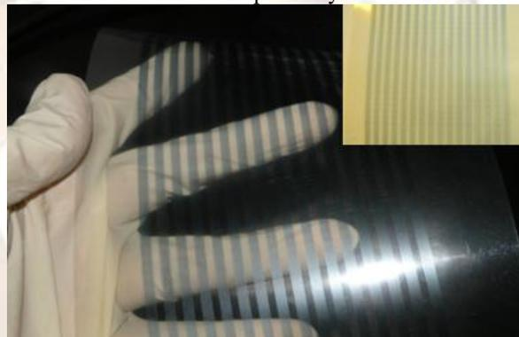
Figure 3 Photograph of PEDOT: PSS coated on PET substrate using slot die process.
